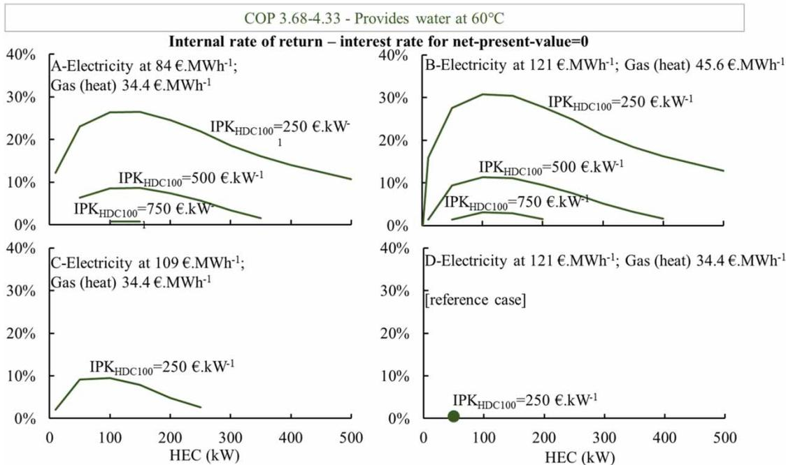
**Figure 4** | Electricity and heat prices effects on the internal rate of return (interest rate for a net-present-value = 0). Electricity prices: 121 €·MWh<sup>-1</sup> (Euro-area year 2017), 109 €·MWh<sup>-1</sup> (2009), 84 €·MWh<sup>-1</sup> (production on site); Gas (heat) prices: 34.4 €·MWh<sup>-1</sup> (2017), 45.6 €·MWh<sup>-1</sup> (2013).
