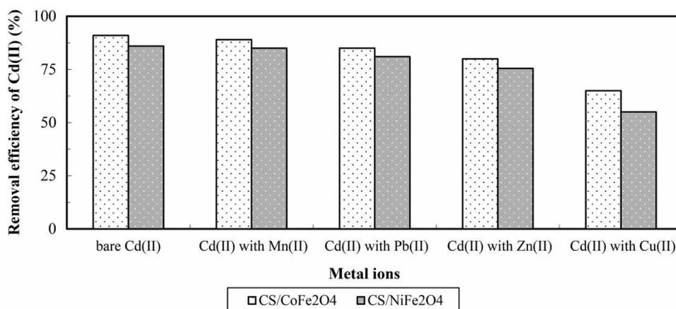
**Figure 4** | Effect of coexisting cations on Cd(II) removal efficiency. Experimental conditions: pH 6.0, 0.05 g of adsorbent, 25 mL of 20.0 mg L<sup>-1</sup> of Cd(II) and coexisting cation in binary solution, and contact time of 60 min.
