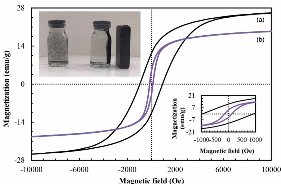
**Figure 2** | Magnetization curves measured at room temperature for (a) CS/ $\text{CoFe}_2\text{O}_4$  and (b) CS/ $\text{NiFe}_2\text{O}_4$ . Insets are magnified views of the hysteresis loops at the low applied field.
