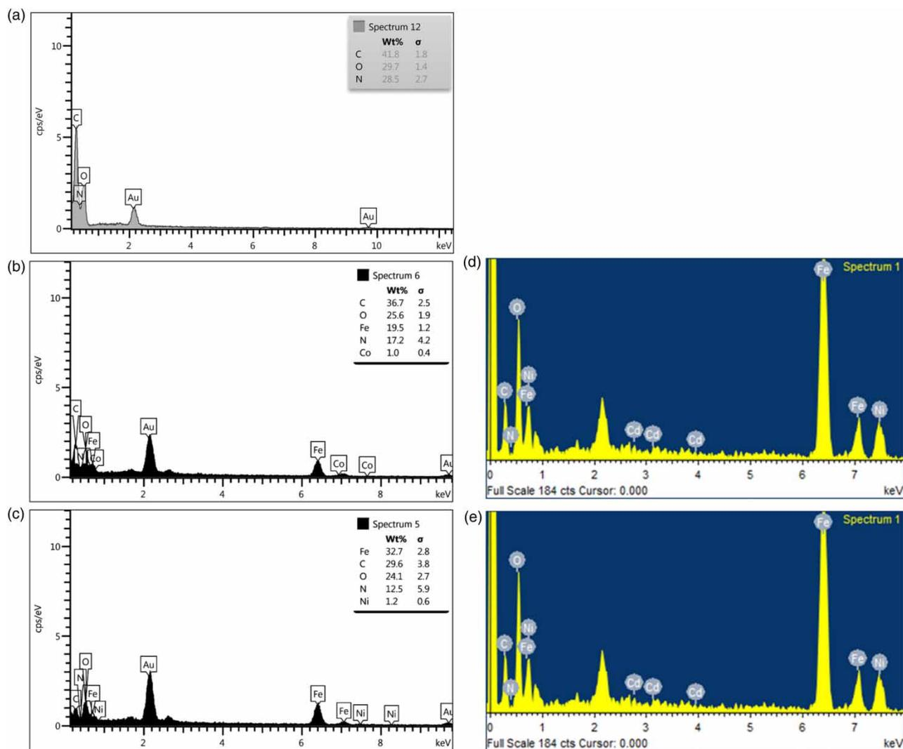
**Figure 1** | The EDX spectra of (a) chitosan, (b) CS/ $\text{CoFe}_2\text{O}_4$ , and (c) CS/ $\text{NiFe}_2\text{O}_4$ ; the EDX spectra of (d) CS/ $\text{CoFe}_2\text{O}_4$  and (e) CS/ $\text{NiFe}_2\text{O}_4$  after Cd(II) ions adsorption.
