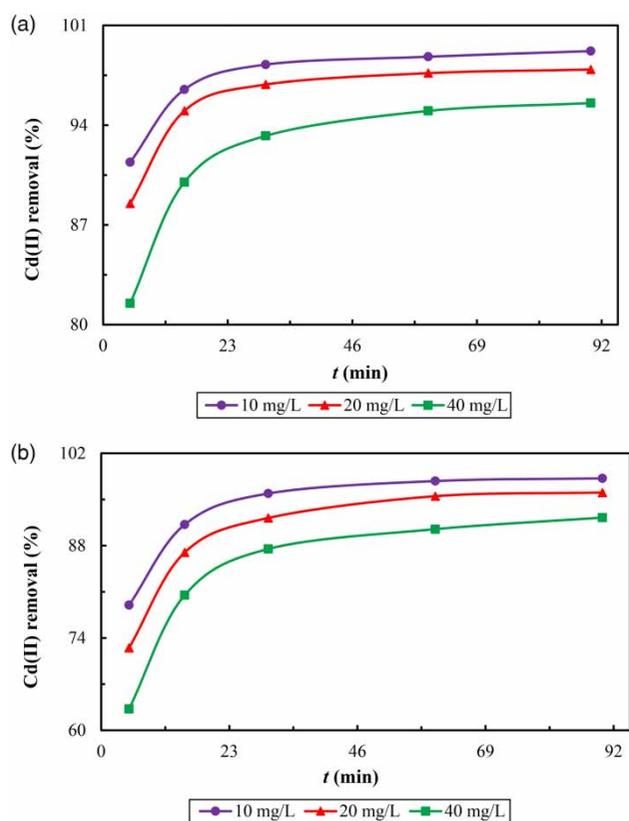
**Figure 3** | Effect of contact time and initial ion concentration on Cd(II) removal efficiency with (a) CS/CoFe<sub>2</sub>O<sub>4</sub> and (b) CS/NiFe<sub>2</sub>O<sub>4</sub>. Experimental conditions: pH 7.0, 0.05 g of adsorbent, 25 mL of Cd(II) solution.
