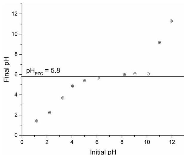
**Figure 1** | Experimental data of pH<sub>PZC</sub> for the adsorbent VAC (160 rpm, 30 °C, adsorbent dose: 1 g/L, contact time: 24 h).
