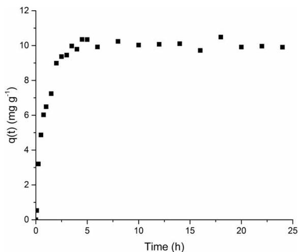
**Figure 4** | Adsorption kinetics of prednisone in VAC (160 rpm, T: 30 °C, adsorbent mass: 0.02 g, V: 50 mL, C<sub>0</sub>: 10 mg/L, pH 6.46).
