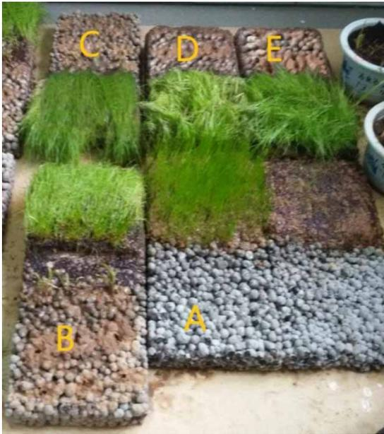
**Figure 2** | Picture showing plant growth ability of the different porous concrete templates.
