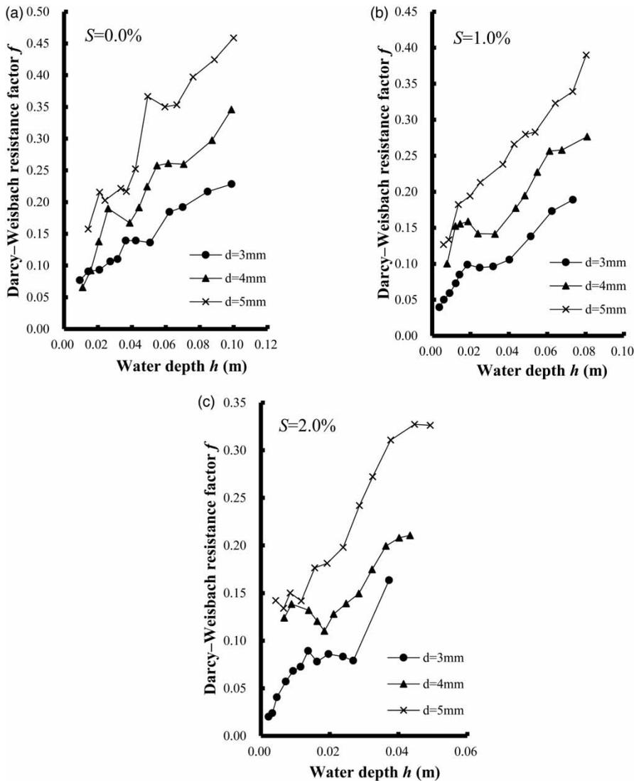
Figure 4 | Curve of Darcy-Weisbach resistance factor  $f$  and water depth  $h$  for three vegetation stem diameters under different slopes gradients.
