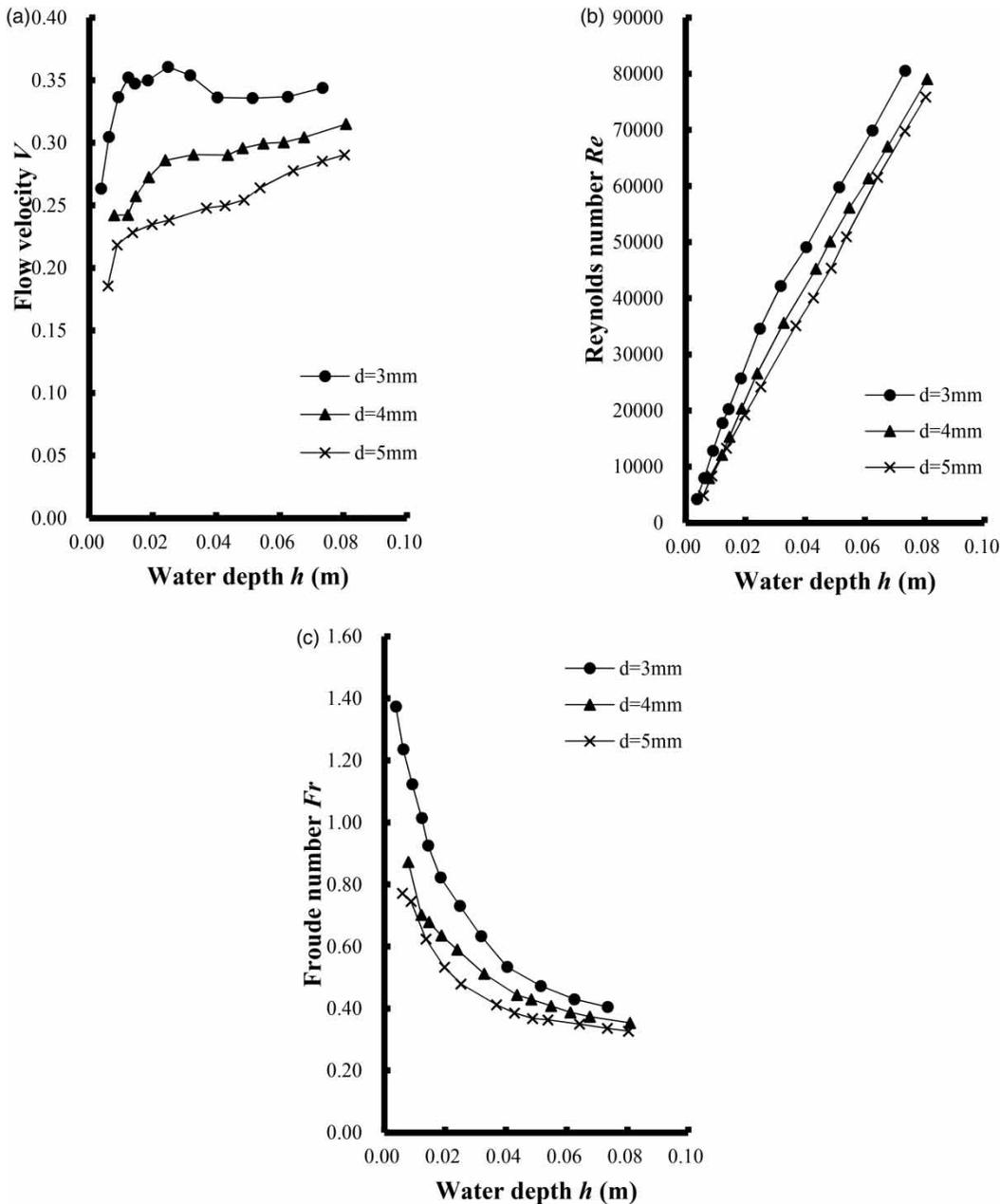
**Figure 5** | Relationships among (a) flow velocity  $V$  versus water depth  $h$ , (b) Reynolds number  $Re$  versus water depth  $h$ , (c) Froude number  $Fr$  versus water depth  $h$  of three vegetation stem diameters under slopes gradient is 1.0%.
