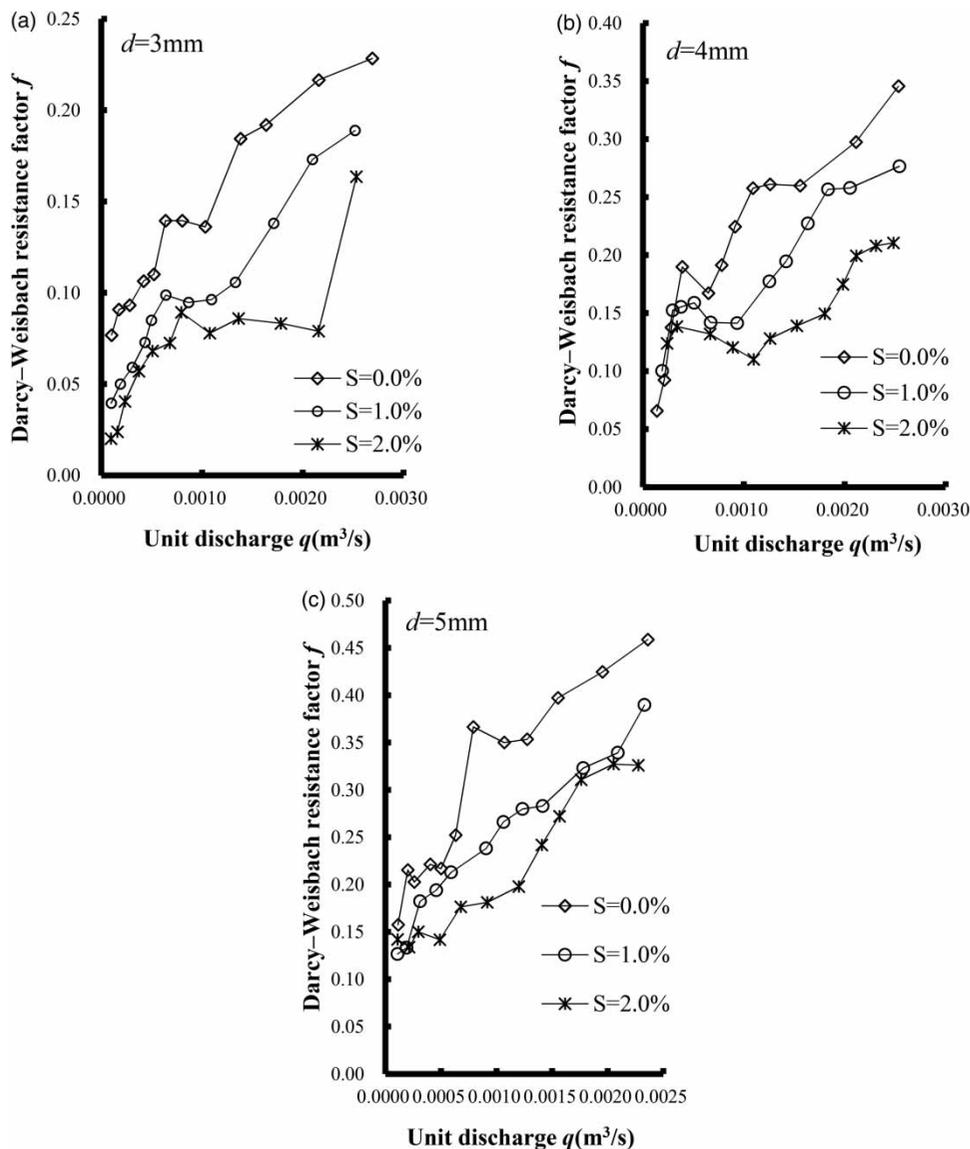
Figure 6 | Curve of Darcy-Weisbach resistance factor  $f$  and unit discharge  $q$  for three slope gradients under different stem diameters.
