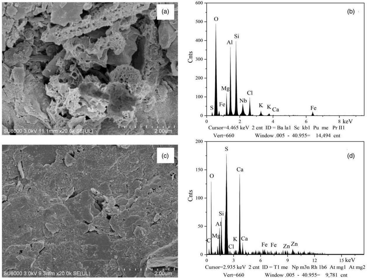
**Figure 3** | SEM micrograph and EDX spectrum of WTPS (a) and (b) and sediment of WTPS mixed with FGD wastewater (c) and (d).
