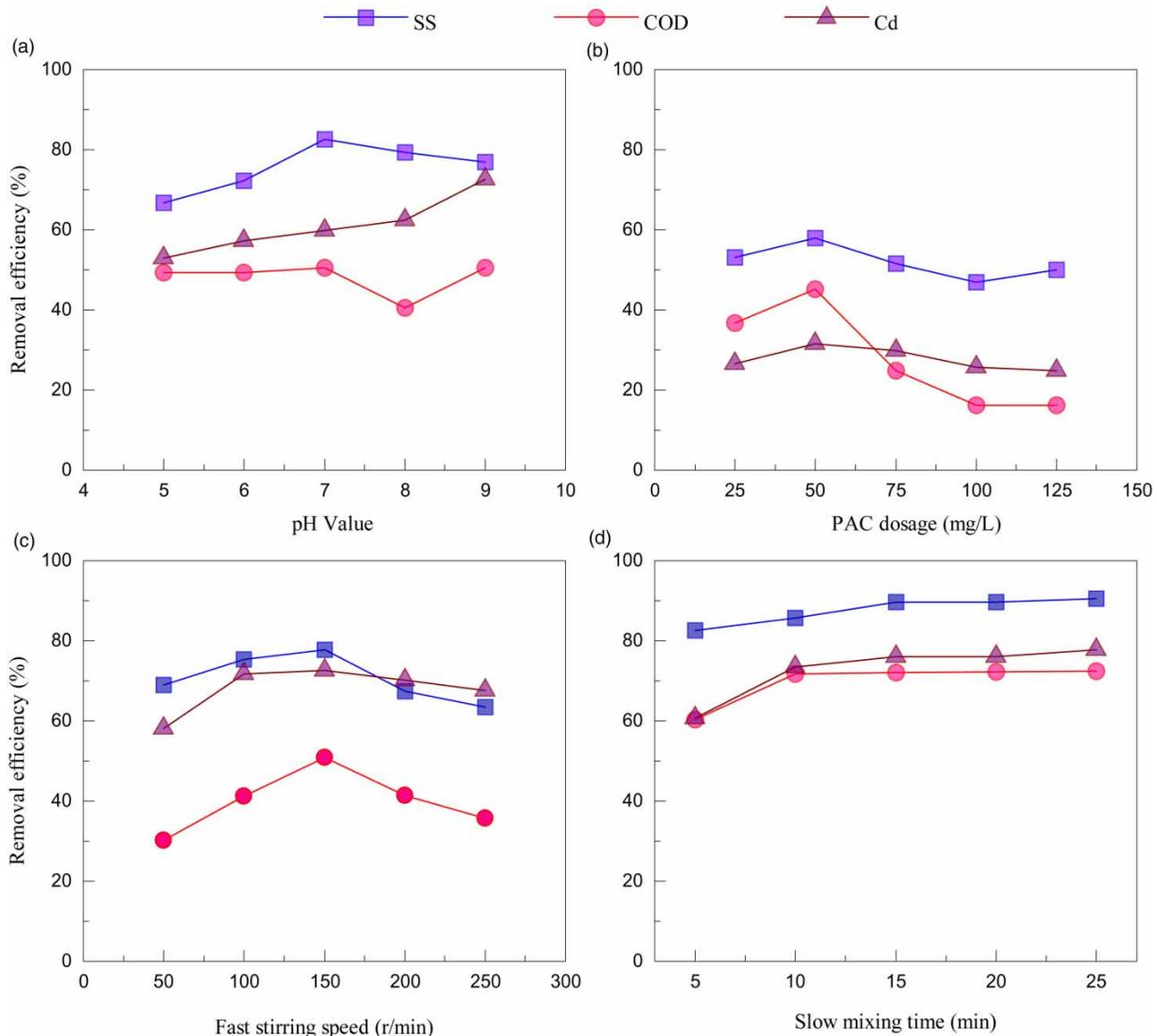
Figure 5 | Advanced treatment of the FGD wastewater by PAC coagulation.
