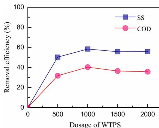
Figure 2 | Effects of WTPS addition on SS and COD removal efficiencies of FGD wastewater.
