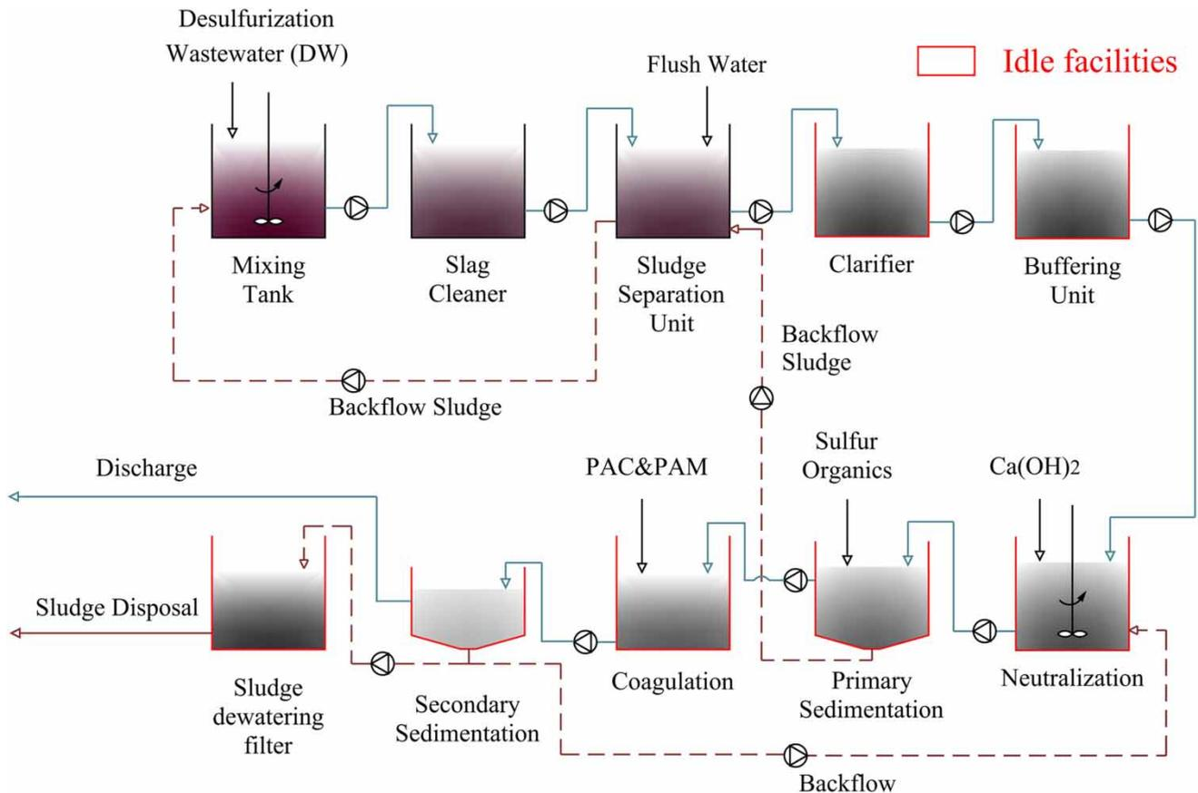
Figure 1 | Flow chart of the existing process for FGD wastewater treatment.
