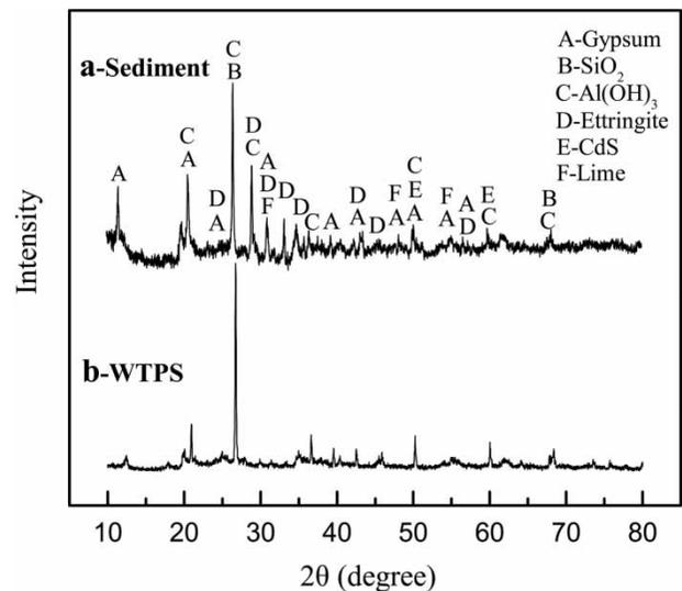
**Figure 4** | XRD pattern of WTPS and sediment of WTPS mixed with FGD wastewater.
