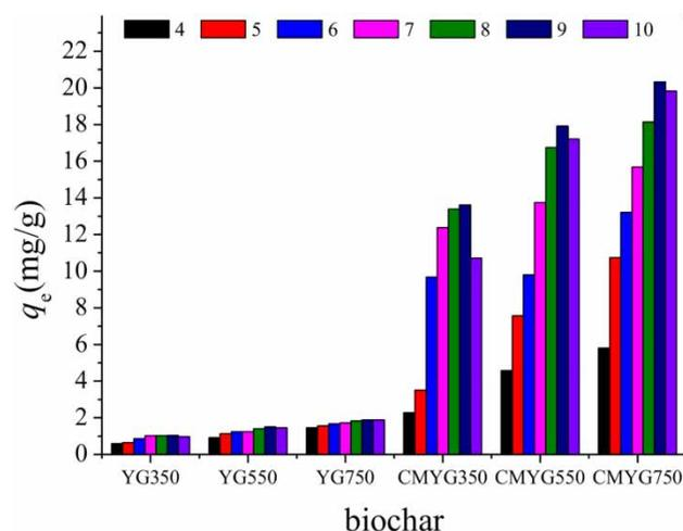
Figure 1 | Effect of the solution pH on YGs and CMYGs adsorption of phosphate.
