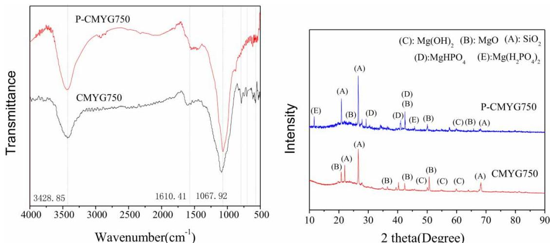
**Figure 2** | FTIR and XRD analyses of CMYG750 and P-CMYG750.
