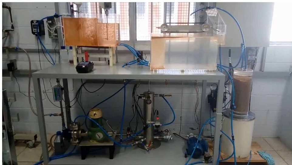
Figure 1 | DAF pilot plant.
