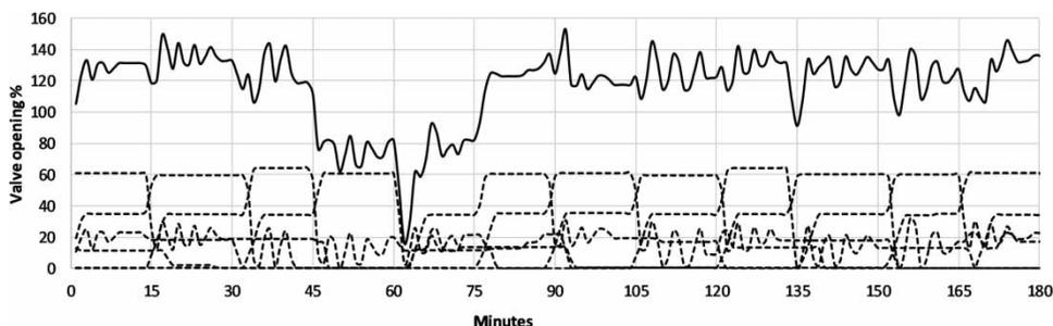
**Figure 6** | Train 2 steam valve position of single batches (dashed lines) and summation of all valve positions (solid line).
