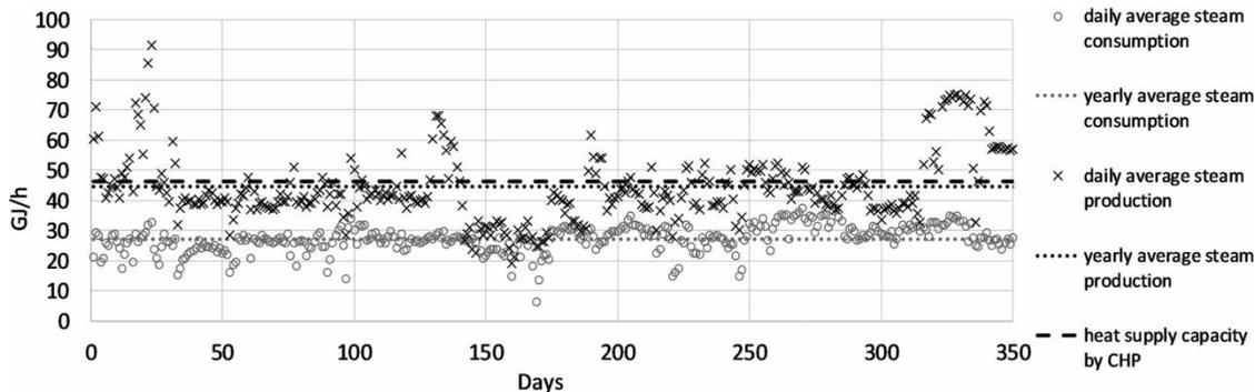
**Figure 5** | Steam production and steam consumption at the THP-system Blue Plains. Supply capacity is limited by the average gas production. Steam production above CHP capacity necessitates duct burner operation.
