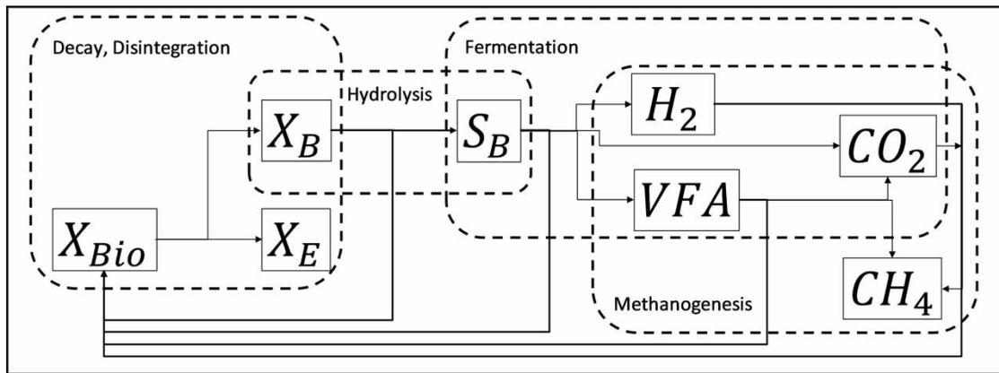
Figure 1 | Process-scheme of anaerobic digestion of biomass.
