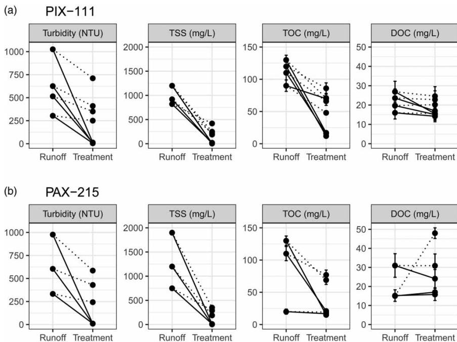
**Figure 1** | Treatment effects for PIX-111 (a) and PAX-215 (b) with respect to particles (turbidity and TSS) and organic carbon (total and dissolved). Solid line (—) represents treatment with a coagulant plus sedimentation, dotted line (···) represents the control (only sedimentation) in the jar tests. Error bars cover two standard deviations from the mean as reported by the laboratory where applicable.
