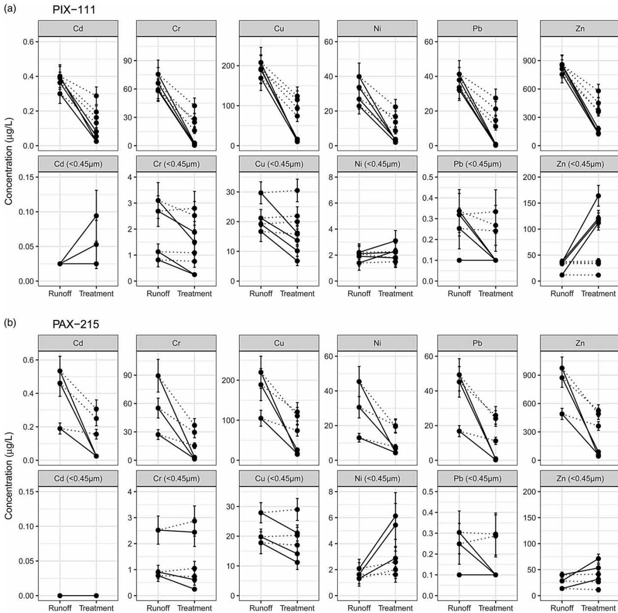
**Figure 2** | Metal treatment effects for road runoff treated with PIX-111 (a) and PAX-215 (b). Solid line (—) represents treatment with a coagulant plus sedimentation, dotted line (---) represents the control (only sedimentation) in the jar tests. Error bars cover two standard deviations from the mean as reported by the laboratory.
