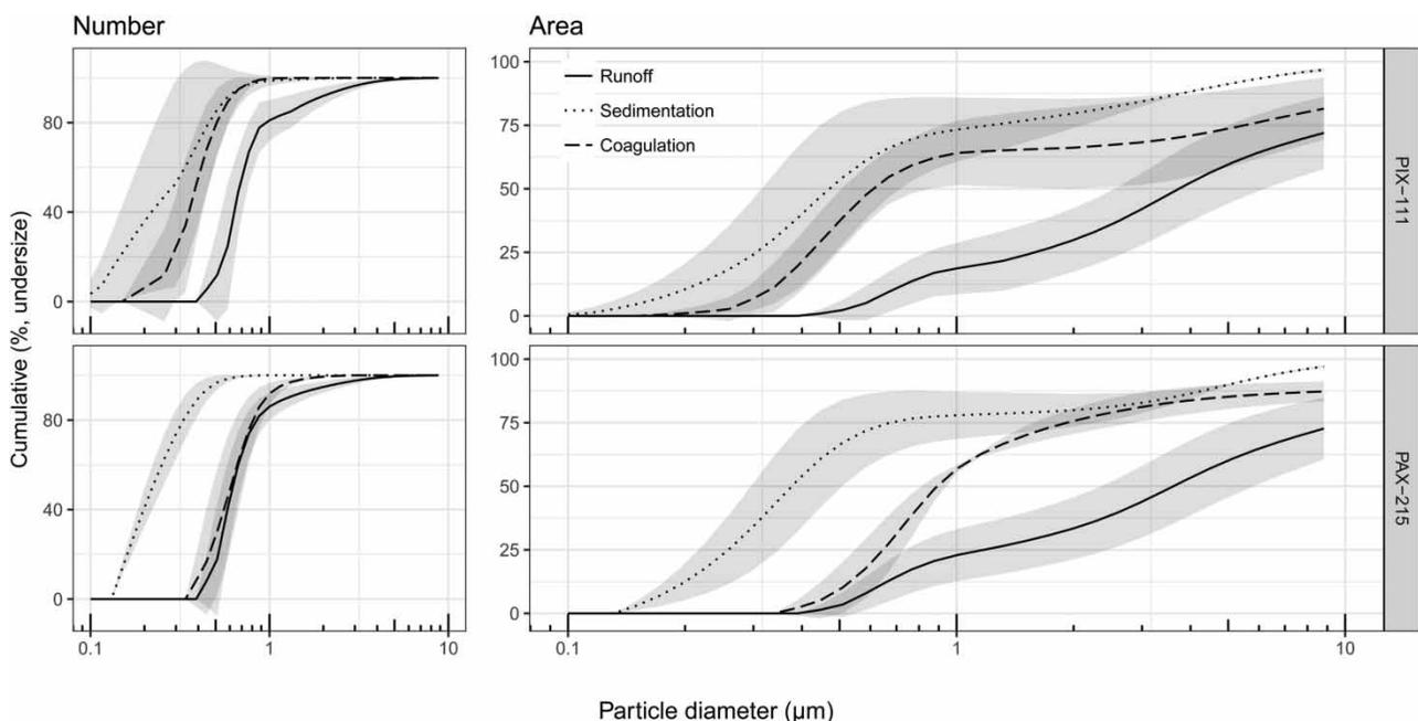
**Figure 3** | Average particle size distribution for the road runoff, and after treatment (sedimentation and coagulation). Left column uses number as its transformation basis and right column uses area. The y-axis represents the cumulative percentage of undersize particles for the given basis. Shaded region includes one standard deviation around the mean.
