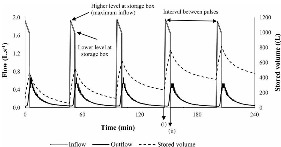
Figure 1 | Inflow, outflow and stored volume inside the filter as a function of time. Five sequential pulse events are represented.
