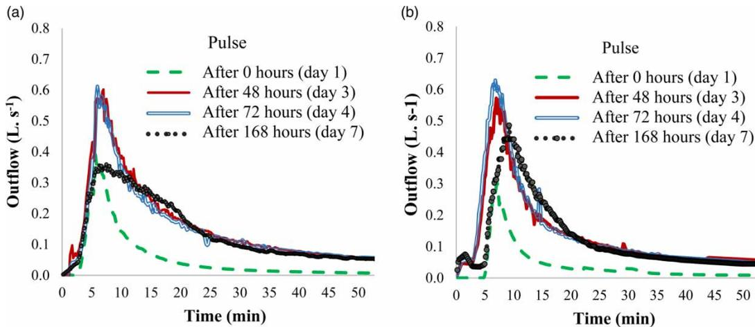
Figure 6 | Outflow hydrographs from different pulses through the seven-day feeding cycle. (a) Unit with sludge layer (left). (b) Unit with sludge layer previously removed (unit displayed in the other graphs) (right).
