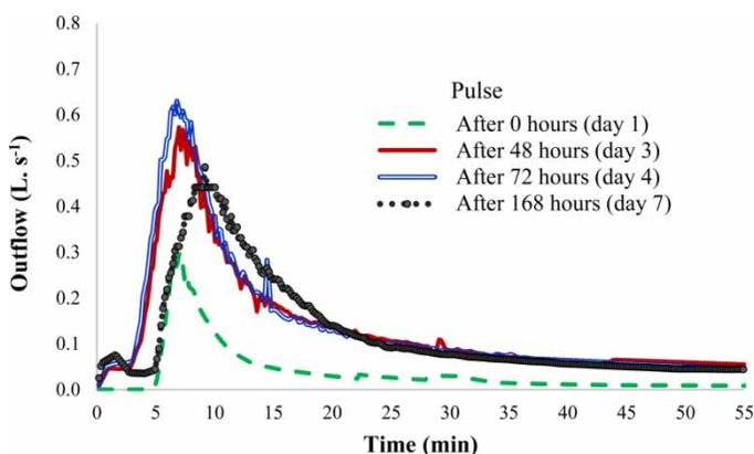
**Figure 2** | Batches (pulses) on different days of one feeding cycle: outflow as a function of time.
