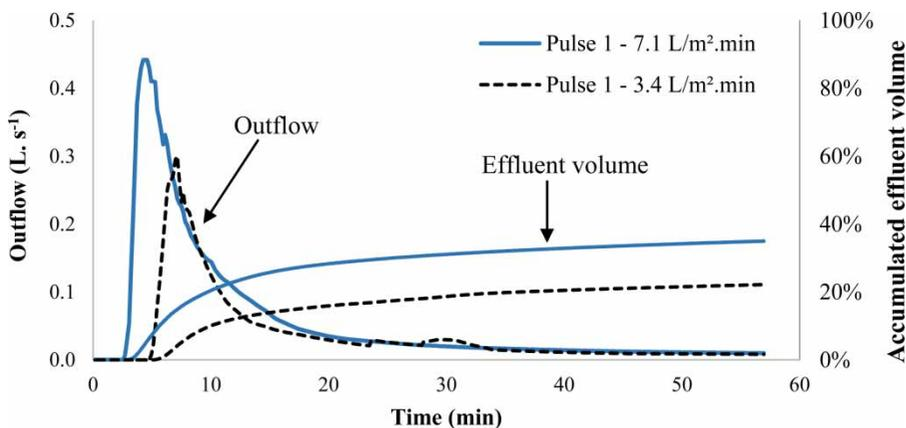
Figure 4 | Difference between instantaneous hydraulic loading rates: outflow and accumulated effluent volume as a function of time (in relation to the applied volume of  $0.55 \text{ m}^3$  in the pulse).
