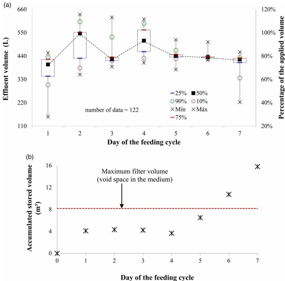
**Figure 3** | (a) Effluent volume and percentage of recovery of the different pulses of each day of the cycle (top). (b) Cumulative volume stored in the filter during each day of the feeding cycle (bottom).
