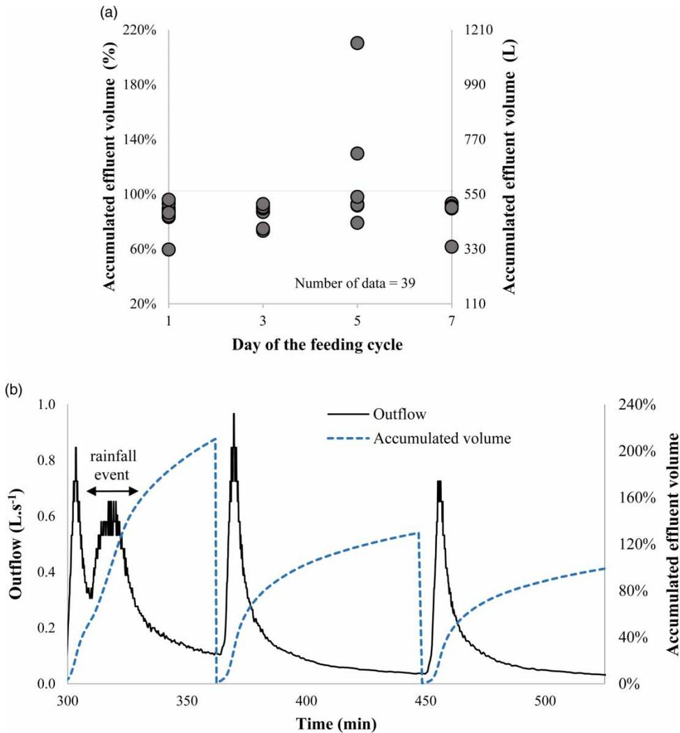
Figure 5 | (a) Effluent volume on the days of the feeding cycle during the rainy period (top). (b) Sequence of pulses during a heavy rain (rainfall event at minutes 300 to 350) (bottom).
