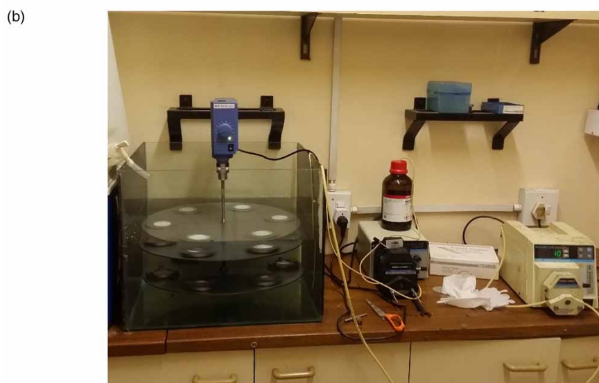
Figure 1 | (a) A typical set-up showing the calibration of MIM-based passive samplers with a flow-through set-up with an overflow to waste. (b) A typical set-up showing the calibration of MIM-PSD passive samplers using a flow-through set-up with an overflow to waste.
