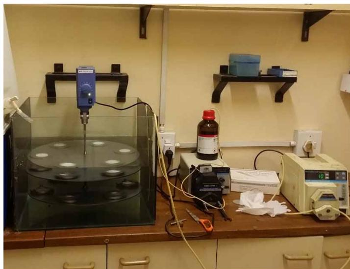
**Figure 1** | (a) A typical set-up showing the calibration of MIM-based passive samplers with a flow-through set-up with an overflow to waste. (b) A typical set-up showing the calibration of MIM-PSD passive samplers using a flow-through set-up with an overflow to waste.
