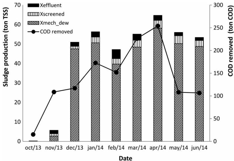
**Figure 2** | The sludge production and the amount of COD removed during the AS + ASSR operation.
