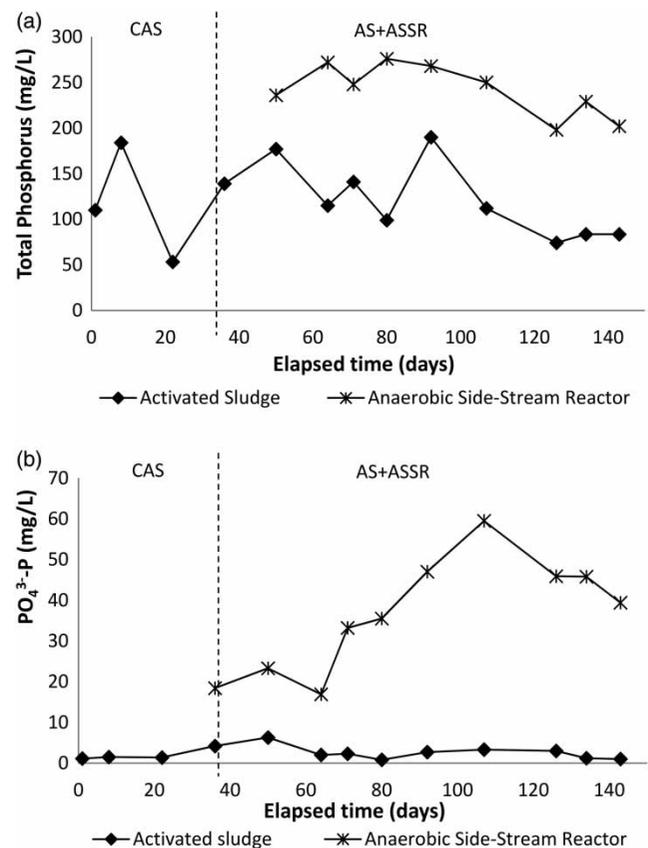
Figure 5 | Time profiles of (a) Total Phosphorus and (b)  $PO_4^{3-}P$  in the sludge samples over the monitored periods.
