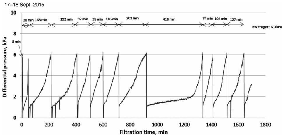
Figure 3 | Online data for pressure drop (BW: backwash).
