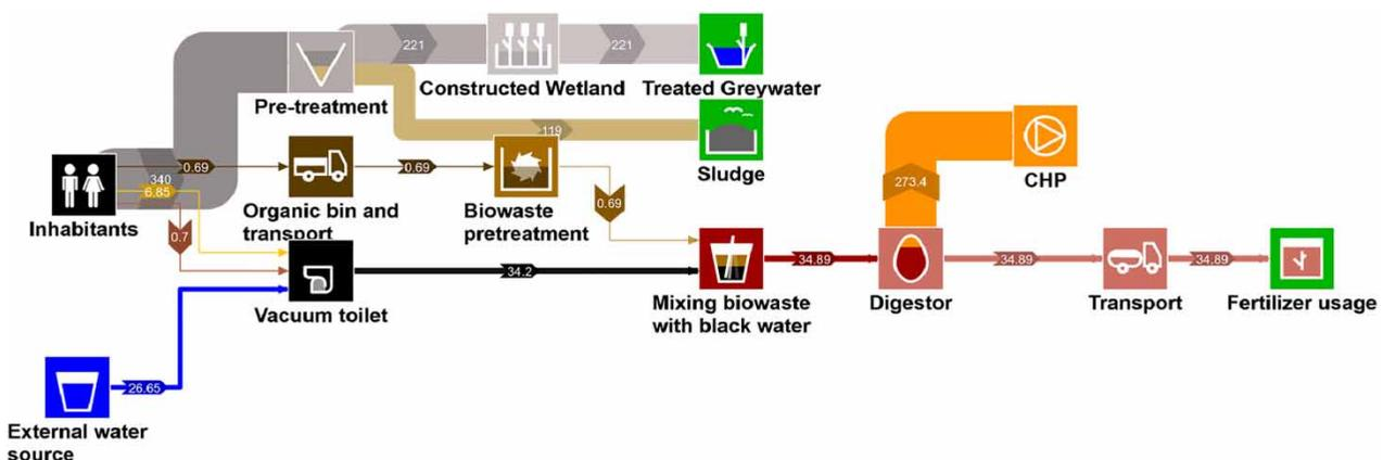
**Figure 6** | Illustration of wastewater flows [m<sup>3</sup>/d] in the scenario with co-digestion of blackwater and separated greywater treatment (N.B. The outputs of the 'Inhabitants' block shown in the figure refer to the biowaste, greywater, urine and faeces fluxes).
