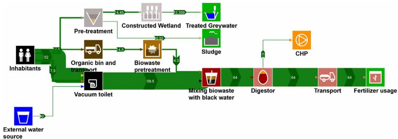
**Figure 7** | Illustration of nitrogen fluxes [kg/d] in the scenario with co-digestion of blackwater and separated greywater treatment.
