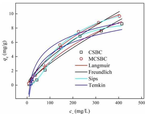
**Figure 5** | Adsorption isotherms of Cr(VI) on CSBC and MCSBC.**Table 3** | Isotherm parameters of Cr(VI) adsorption on CSBC and MCSBC
