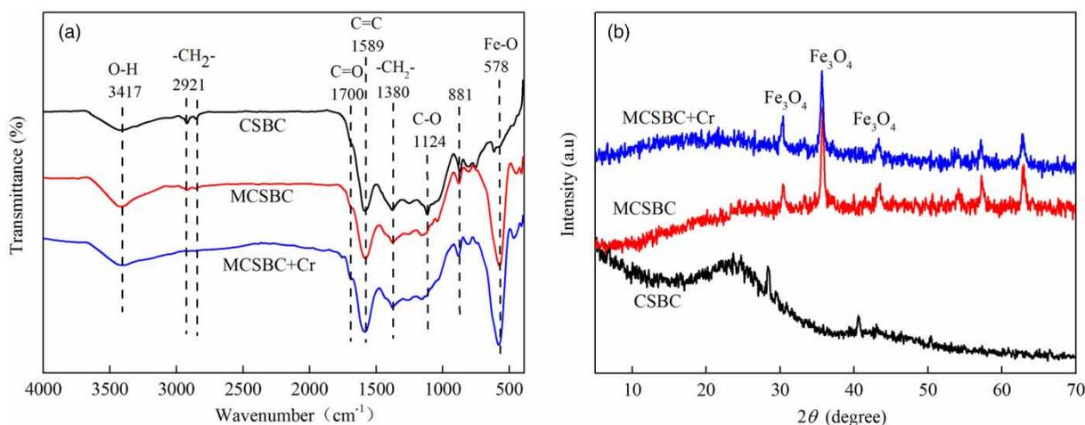
**Figure 1** | FTIR spectrum (a) and XRD pattern (b) of CSBC, MCSBC, and MCSBC with Cr(VI) adsorption.
