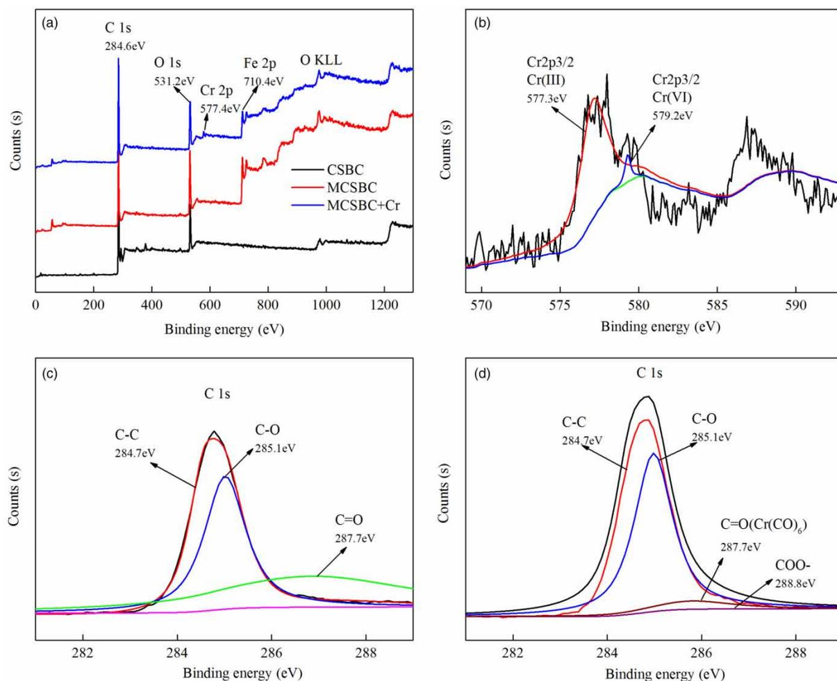
**Figure 2** | (a) XPS spectrum of CSBC, MCSBC, and MCSBC with Cr(VI) adsorption; (b) deconvolution of Cr 2p of MCSBC with Cr(VI) adsorption; (c) C 1s of MCSBC; (d) C 1s of MCSBC with Cr(VI) adsorption.
