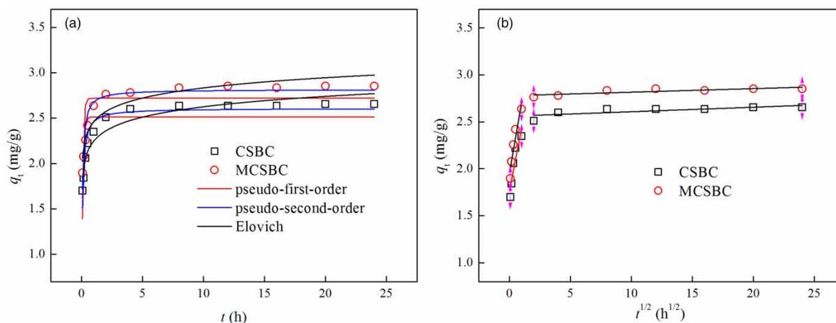
**Figure 4** | (a) Fitting of Elovich, pseudo-first- and pseudo-second-order models for adsorption of Cr(VI) on CSBC and MCSBC. (b) Intra-particle diffusion plots for adsorption of Cr(VI) on CSBC and MCSBC.
