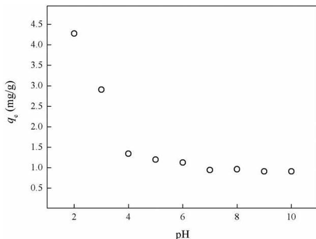
**Figure 6** | Effect of the pH value of the solution on Cr(VI) adsorption on MCSBC.
