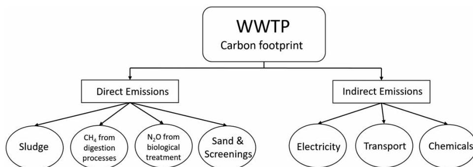
Figure 1 | Direct and indirect emissions discharged from WWTPs.
