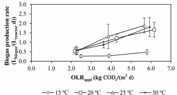
**Figure 5** | Average biogas production rate of the four UASB reactors operated at three OLR<sub>appl</sub>.
