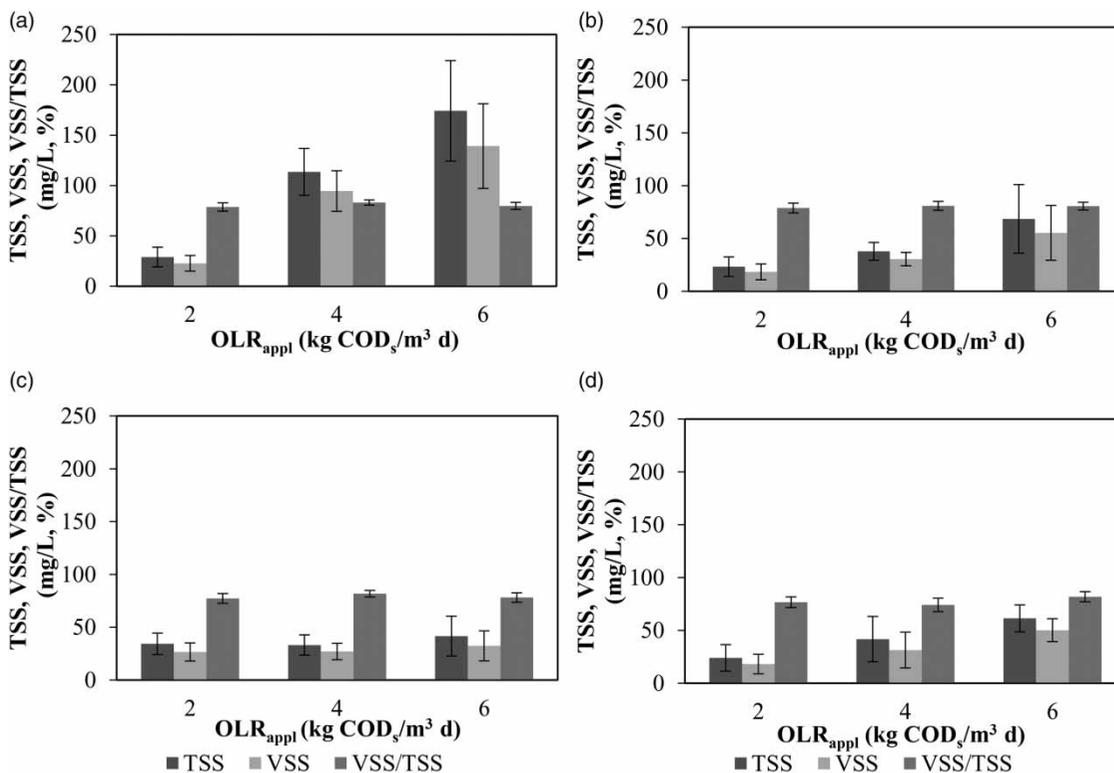
**Figure 2** | The total suspended solids (TSS), volatile suspended solids (VSS) and VSS/TSS ratio of the effluent of UASB reactors: (a) 15 °C, (b) 20 °C, (c) 25 °C and (d) 30 °C.
