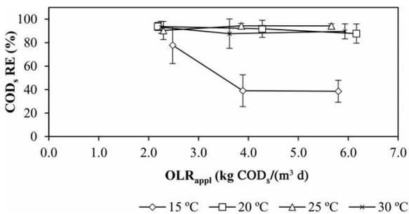
**Figure 4** | COD<sub>s</sub> removal efficiency (RE) of four reactors by OLR<sub>appl</sub>.
