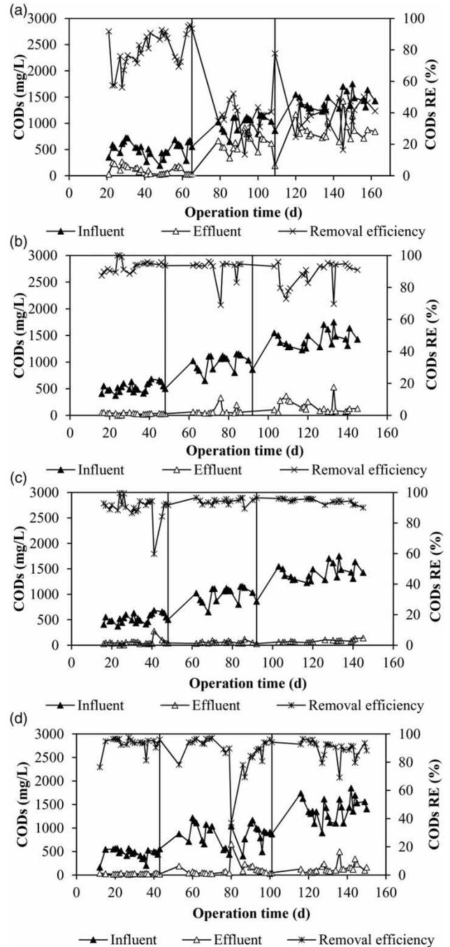
**Figure 3** | The COD<sub>s</sub> removal efficiency (RE) and influent and effluent COD<sub>s</sub> of four laboratory-scale UASB reactors operated at three  $OLR_{appl}$  (2, 4 and 6 kg COD<sub>s</sub>/(m<sup>3</sup> d)) and different operating temperatures: (a) 15 °C, (b) 20 °C, (c) 25 °C and (d) 30 °C. Vertical lines indicate the transition between  $OLR_{appl}$ .
