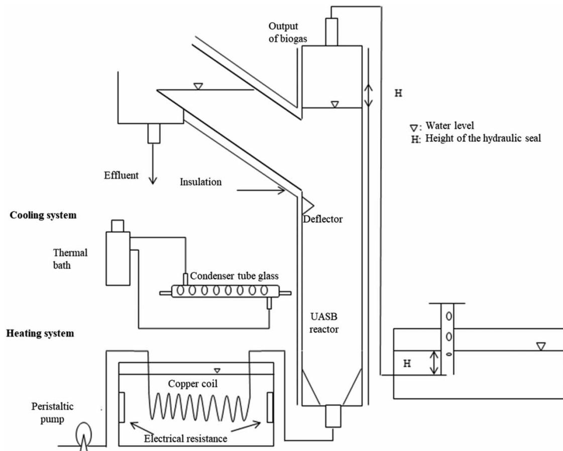
Figure 1 | Scheme of the treatment system of the chocolate-processing industry wastewater.
