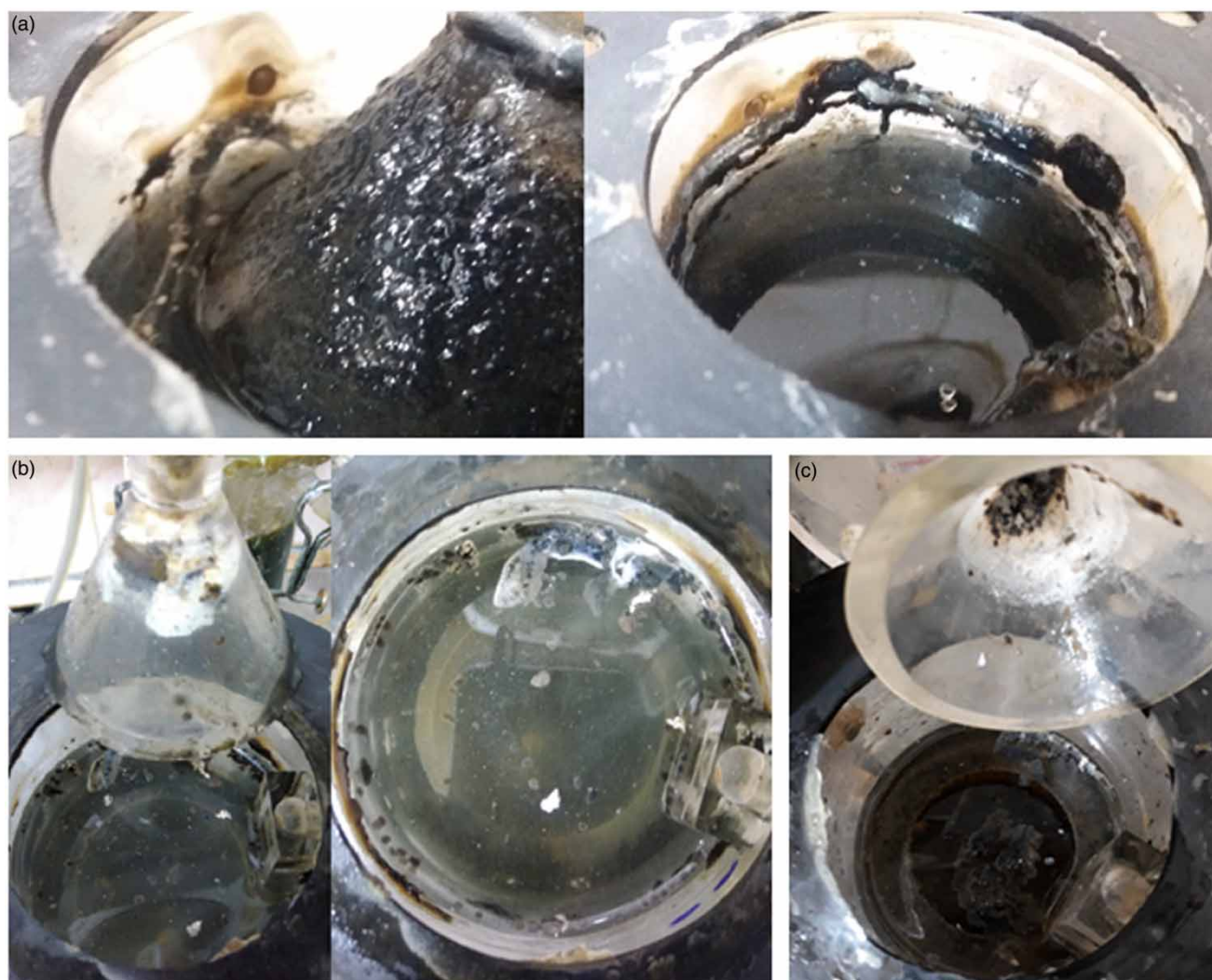
Figure 2 | Aspect of the UASB reactors' top in different phases of operation. (a) Scum deposited on the GLSS device of one of the reactors after 226 days of feeding without addition of enzyme (first phase). (b) GLSS device and surface of the Test reactor (with addition of enzyme in the feed) at 69th day of operation (second phase). (c) Internal part of the GLSS device and surface of the Control reactor (without addition of enzyme in the feed) at 132nd day of operation (second phase).
