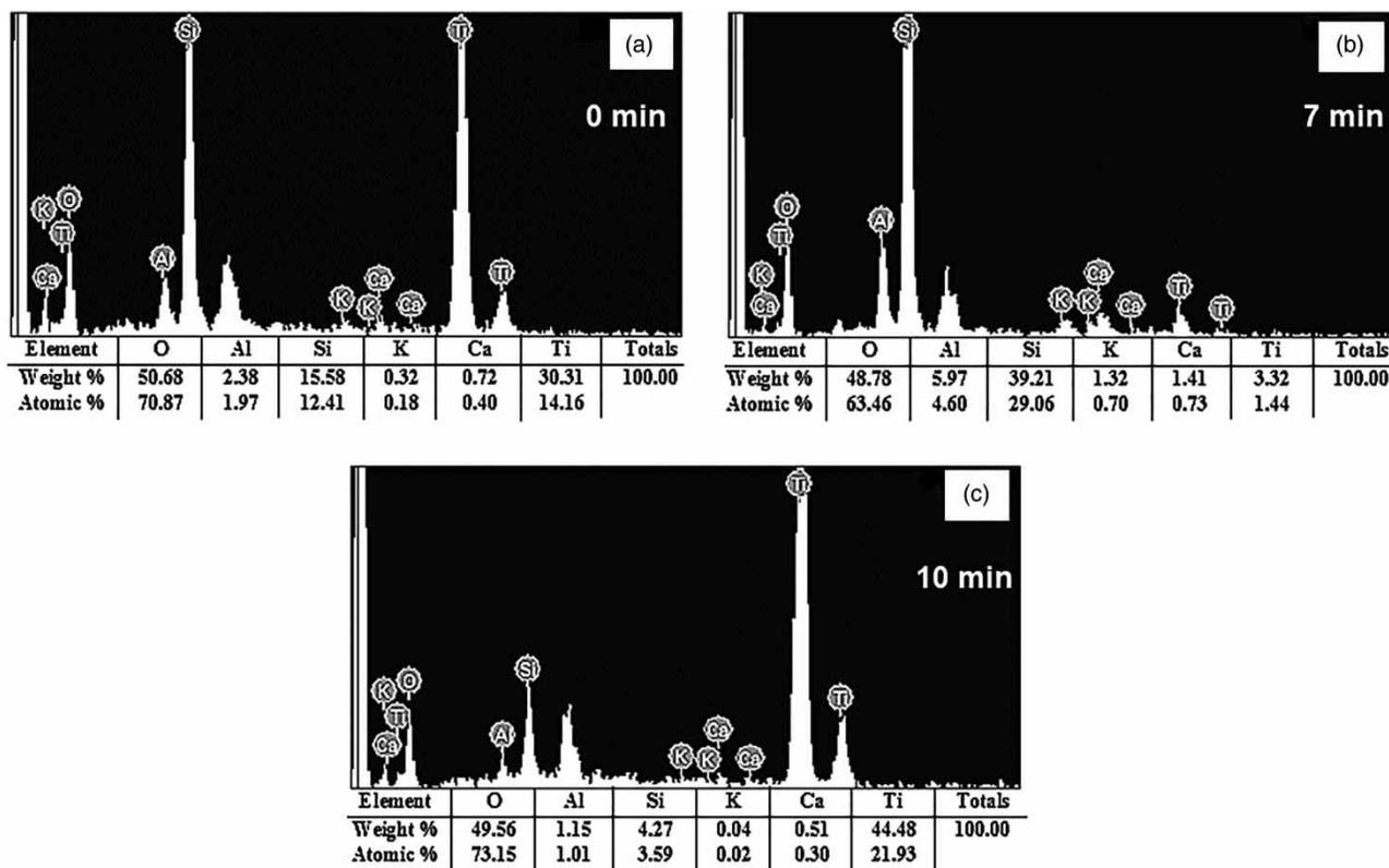
**Figure 6** | EDX images at different irradiation times (a)  $t = 0$ , (b)  $t = 7$  and (c)  $t = 10$  min.
