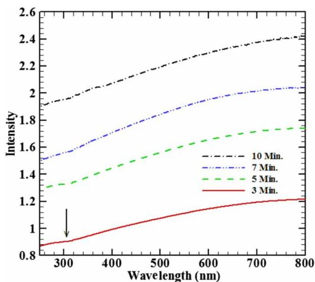
Figure 4 | UV-Vis absorption spectra of the nanocomposite at different laser irradiation times.
