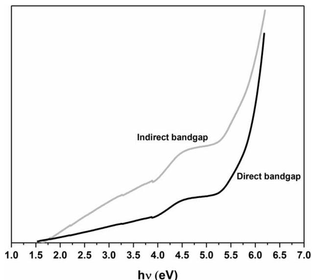
**Figure 8** | Direct (green) and indirect (red) optical band gap of  $\text{TiO}_2$ -Zeolite nanocomposite. Please refer to the online version of this paper to see this figure in colour: <http://dx.doi.org/10.2166/wst.2019.333>.
