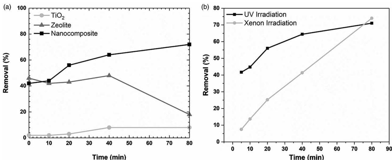
**Figure 7** | (a) Removal of the 2,4-D by nanocomposite, pure Zeolite, and pure TiO<sub>2</sub> under UV irradiation; (b) comparison of 2,4-D removal by the nanocomposite under UV and Xe irradiation at different times.
