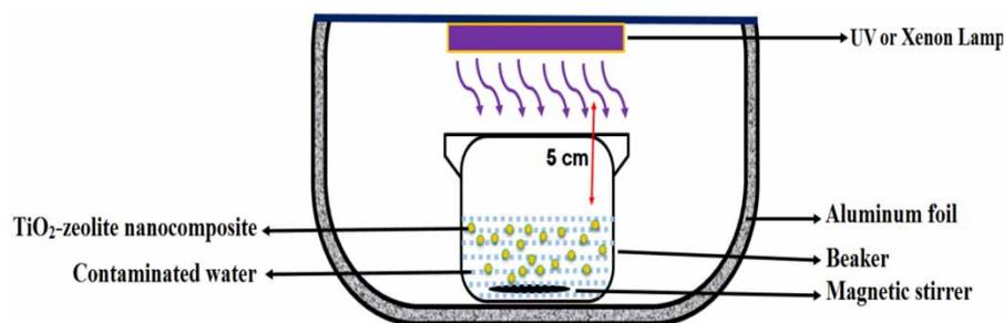
**Figure 1** | Schematic of laboratory-designed photodegradation reactor.
