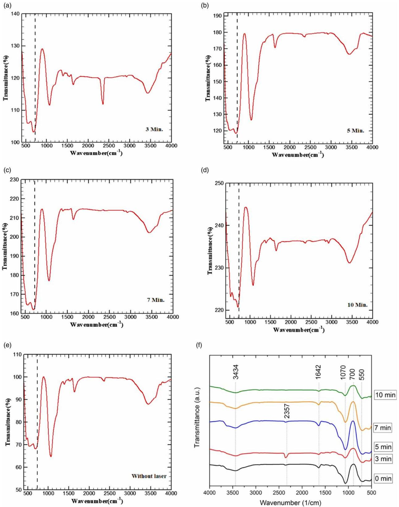
**Figure 2** | FTIR spectra of the sample with: (a) 3, (b) 5, (c) 7, (d) 10, and (e) 0 min laser irradiation; (f) comparison of all the nanocomposites.
