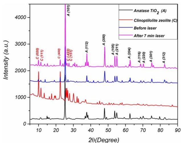
Figure 3 | XRD spectrum of the synthesized nanocomposite at  $t = 0$  and  $t = 7$  min laser irradiation (532 nm).
