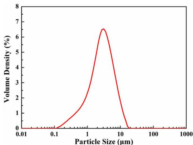
**Figure 2** | The particle size distribution of kaolin.
