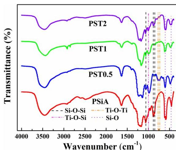
**Figure 4** | FT-IR spectra of PSiA and PST with different Ti/Si molar ratios.
