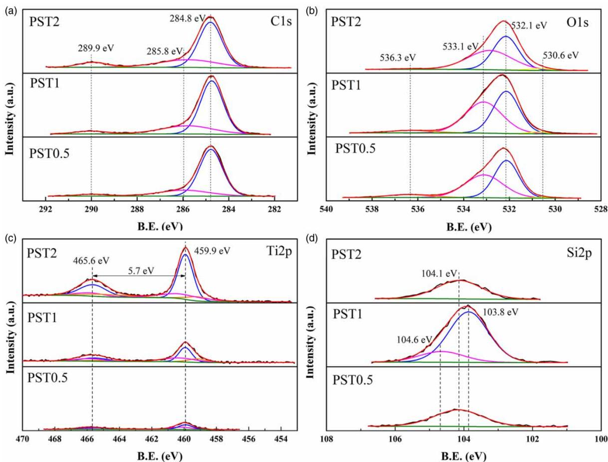
**Figure 5** | XPS spectrum of (a) C1s, (b) O1s, (c) Ti2p XPS and (d) Si2p for the prepared PST (the red line represents the fitted line, the black line represents the original line, the green line represents the baseline, others are the fitting lines). Please refer to the online version of this paper to see this figure in color: <http://dx.doi.org/10.2166/wst.2019.383>.
