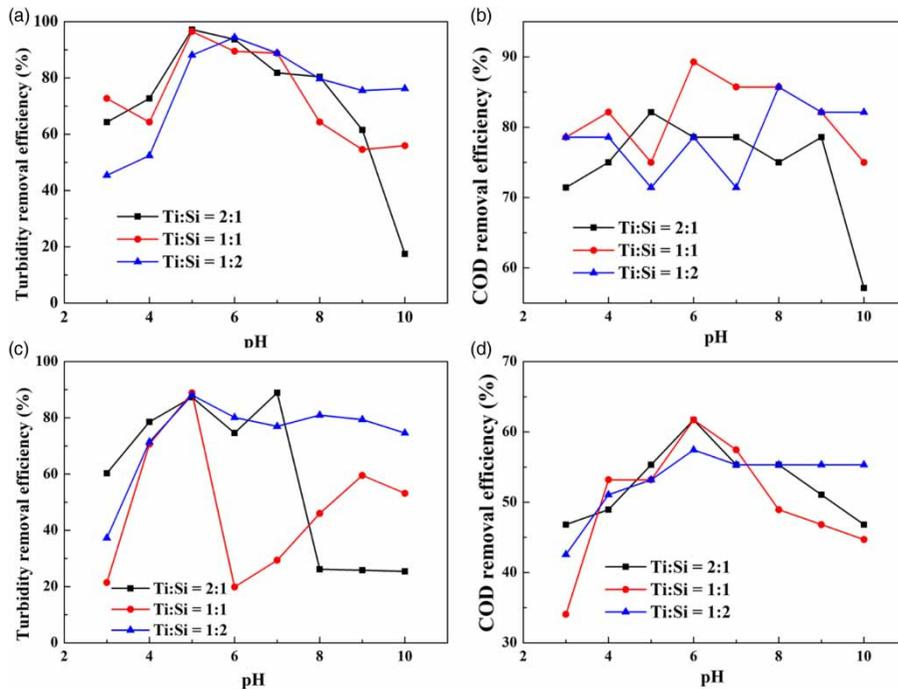
**Figure 6** | Effect of solution pH on PST flocculation performance of PST2, PST1 and PST0.5: (a) turbidity removal rate and (b) COD removal rate of sodium humate–kaolin synthetic water; (c) the turbidity removal rate and (d) COD removal rate of domestic wastewater.
