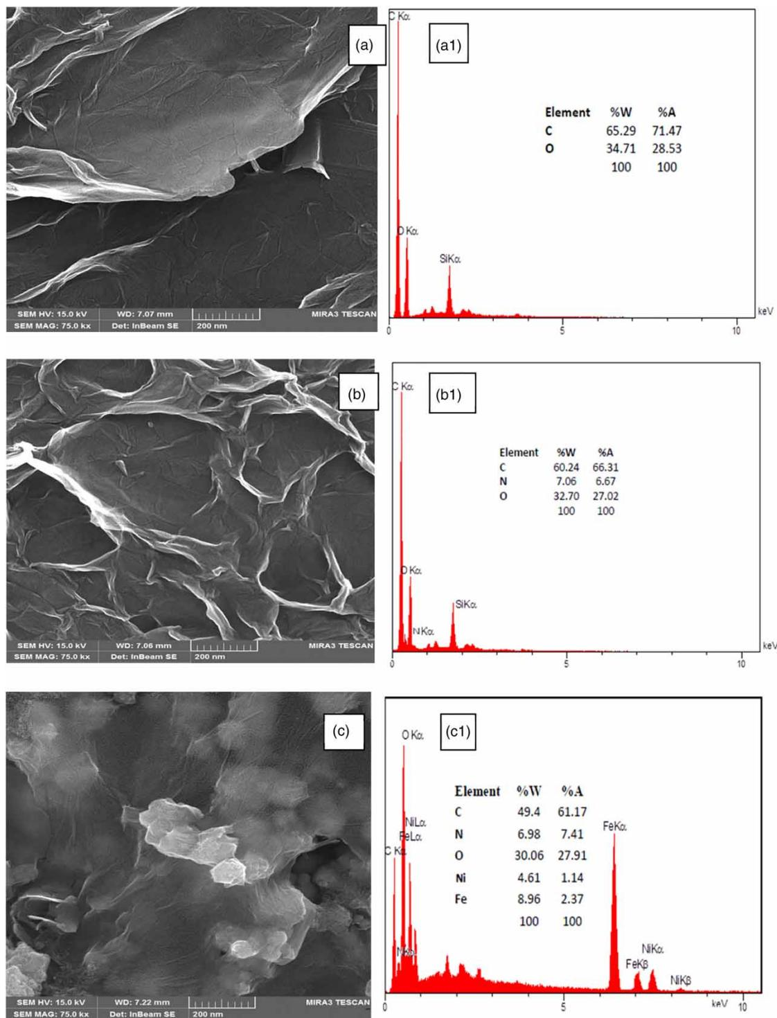
**Figure 1** | SEM images of (a) GO, (b) Ne-GO and (c) NiFe<sub>2</sub>O<sub>4</sub>-Ne-GO nano-particles. EDS spectrum of (a1) GO, (b1) Ne-GO and (c1) NiFe<sub>2</sub>O<sub>4</sub>-Ne-GO.
