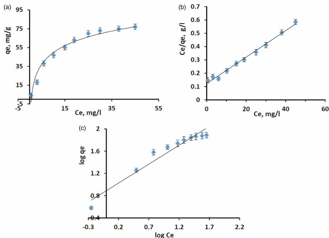
**Figure 6** | Adsorption isotherms for removal of 4-NP using MMNC: (a) Langmuir model, (b) linearized Langmuir and (c) Freundlich model.
