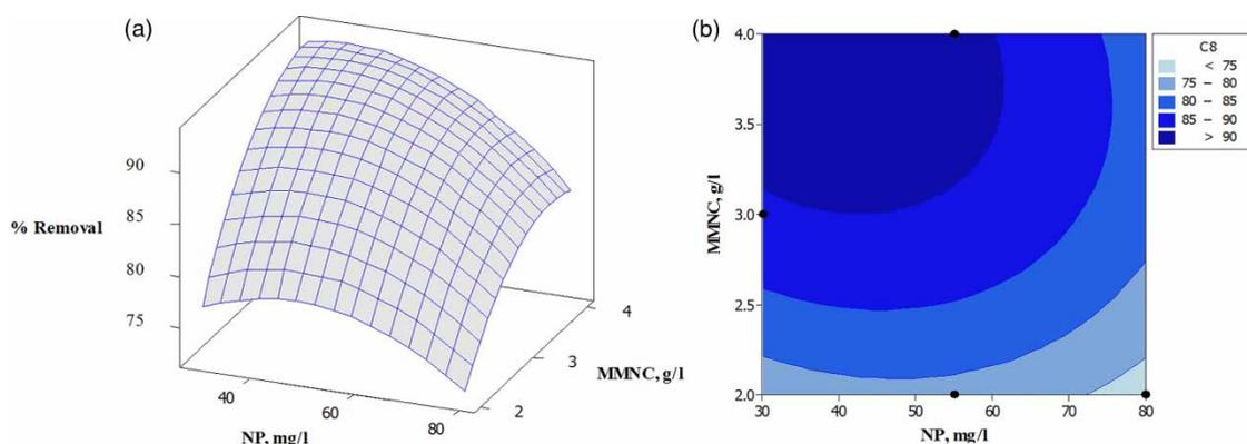
**Figure 3** | Response surface (a) and the corresponding contour (b) plots for removal of 4-NP as function MMNC and 4-NP concentration.
