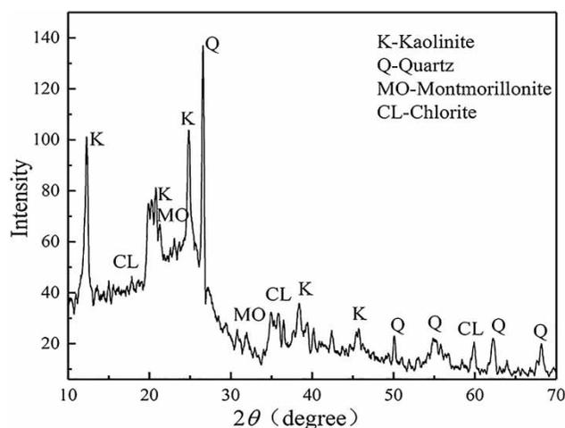
Figure 1 | XRD pattern of coal slurry.
