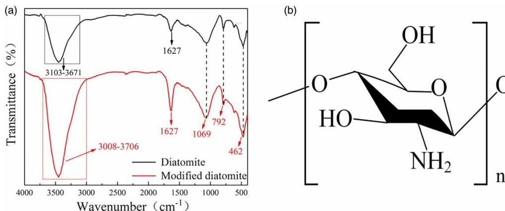
Figure 6 | Infrared spectra of diatomite and modified diatomite (a); molecular structure of chitosan (b).
