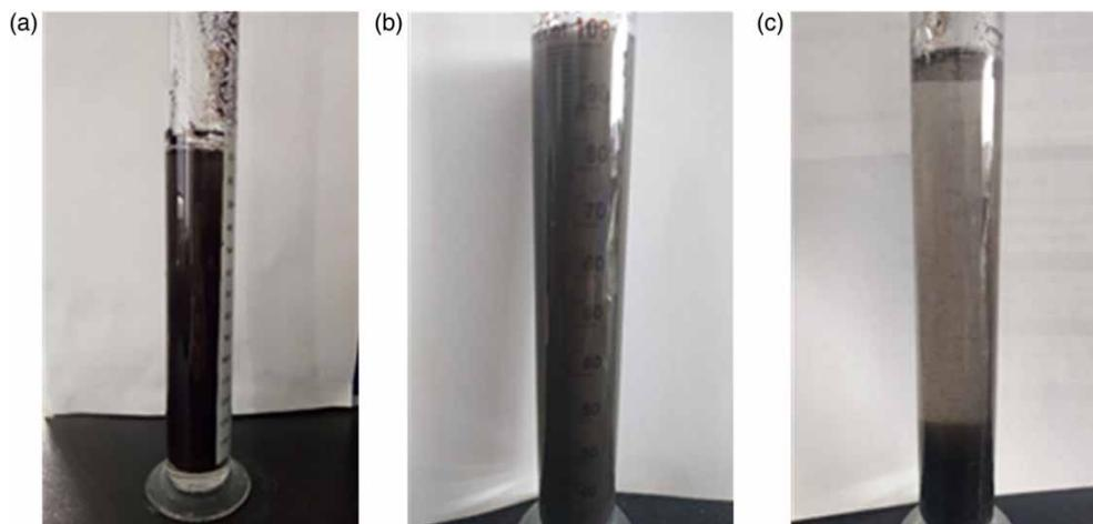
Figure 5 | Settlement effect of different coagulation conditions: natural settling (a); CaCl<sub>2</sub> as a coagulant (b); modified diatomite as coagulant (c).
