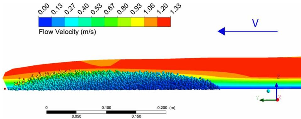
Figure 6 | Velocity of the wave on the middle section plane for the case  $k=0$ ,  $m=1,500$  g,  $h=170$  mm.
