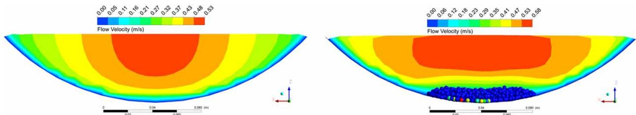
**Figure 4** | Longitudinal flow velocities in a cross section without sediment (left) and in a cross section with sediment (right) for the case  $k = 0$ ,  $d_{50} = 4.33$  mm and a flow rate of 4 l/s.
