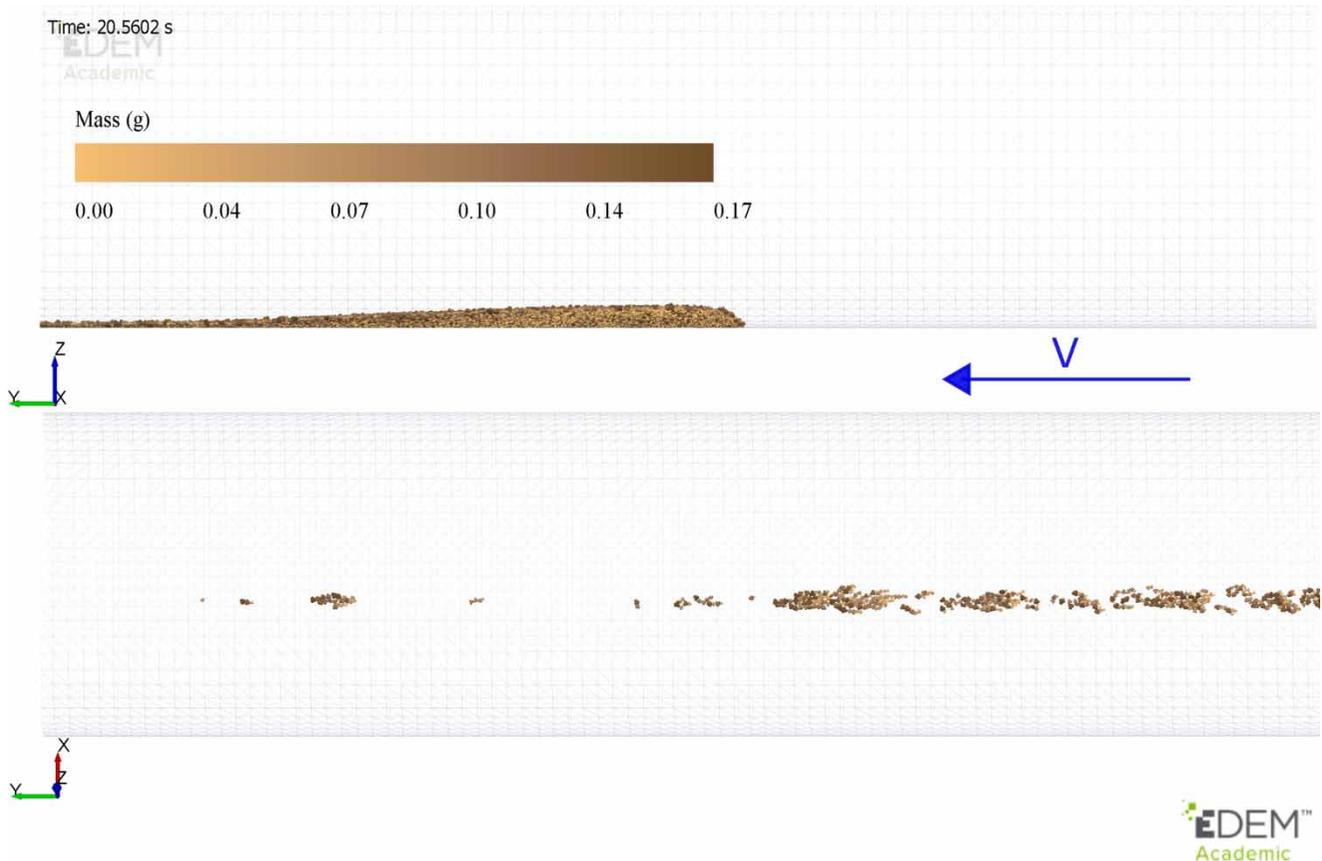
**Figure 5** | Side view of the sediment bed (above) and top view of the scattered sediment at the end of the pipe (down) after the flush in DEM model for the case  $k = 0$ ,  $m = 1,500$  g,  $h = 170$  mm.
