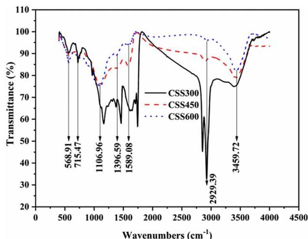
**Figure 2** | FTIR spectra of CSS300, CSS450 and CSS600.
