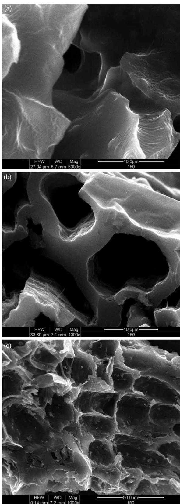
**Figure 1** | The SEM images of (a) CSS300, (b) CSS450 and (c) CSS600.
