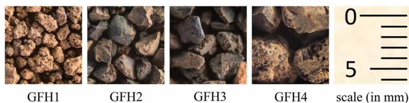
Figure 2 | Macro photographs of the different GFH adsorbents.
