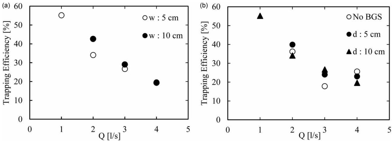
**Figure 6** | (a) Sediment trapping efficiency for cell depths of 5 and 10 cm, and the cross-wall angle of 90°; (b) sediment trapping efficiency for no BGS, a cell width of 5 cm, two depths (5 and 10 cm), and a cross-wall angle of 90°.
