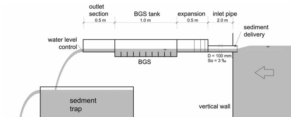
Figure 1 | Experimental setup of the BGS model.
