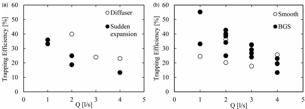
**Figure 4** | (a) Sediment trapping efficiencies with and without the diffuser (cell width and depth 5 cm, cross-wall angle 90°) and (b) sediment trapping efficiencies in runs with and without BGS (smooth bottom runs).
