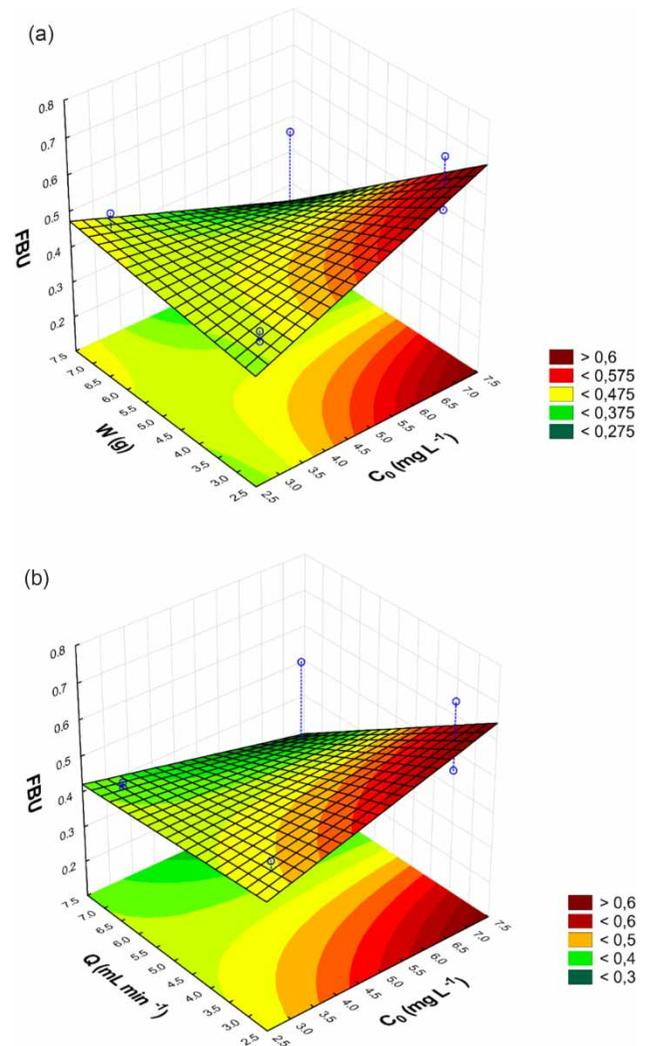
**Figure 7** | Surface responses of the fractional bed utilization of fixed-bed boron adsorption onto activated carbon as function of: (a) initial boron concentration and adsorbent weight ( $Q = 5$  mL min<sup>-1</sup>) and (b) initial concentration and flow rate ( $W = 5$  g).
