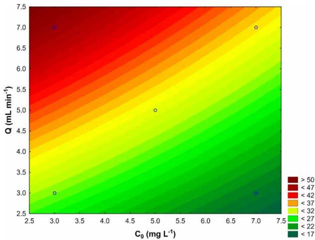
**Figure 6** | Contour plot of the volume of effluent treated by the initial concentration of boron and flow rate ( $W = 5$  g).
