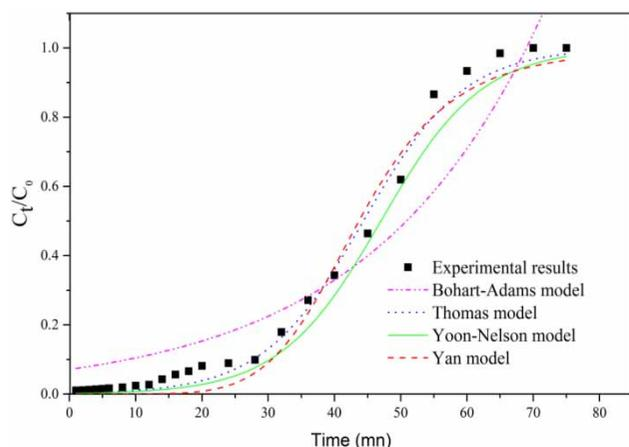
**Figure 8** | Breakthrough curve of boron adsorption onto activated carbon in fixed-bed column ( $C_0 = 3 \text{ mg L}^{-1}$ ,  $W = 7 \text{ g}$ ,  $Q = 3 \text{ mL mn}^{-1}$ ).
