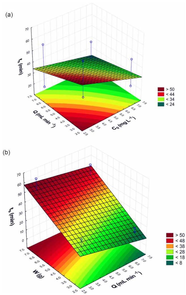
**Figure 5** | Response surfaces of the saturation time of fixed-bed boron adsorption onto activated carbon as function of: (a) initial boron concentration and flow rate ( $W = 5$  g); and (b) adsorbent weight and flow rate ( $C_0 = 5$  mg L<sup>-1</sup>).
