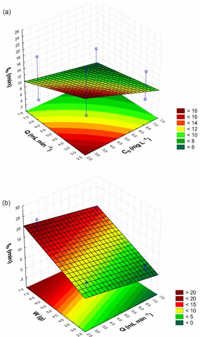
**Figure 4** | Response surfaces of the breakthrough time of fixed-bed boron adsorption onto activated carbon as function of: (a) initial boron concentration and flow rate ( $W = 5$  g); and (b) adsorbent dosage and flow rate ( $C_0 = 5$  mg L<sup>-1</sup>).
