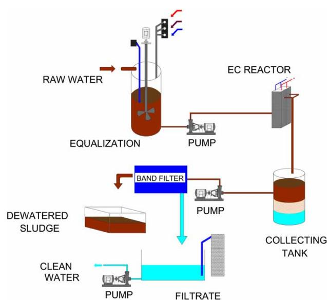
Figure 1 | Wastewater treatment plant with EC process.
