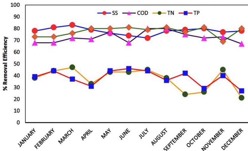
Figure 8 | Pollutant removal efficiencies of the EC process.
