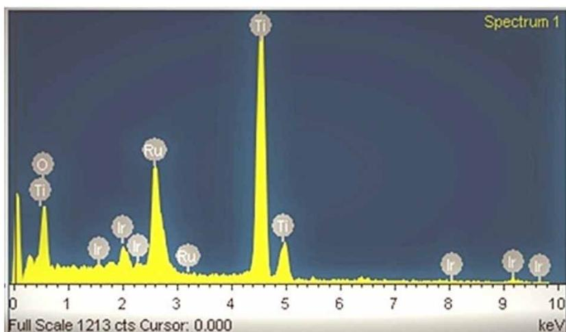
**Figure 5** | EDS image of MMO electrode.
