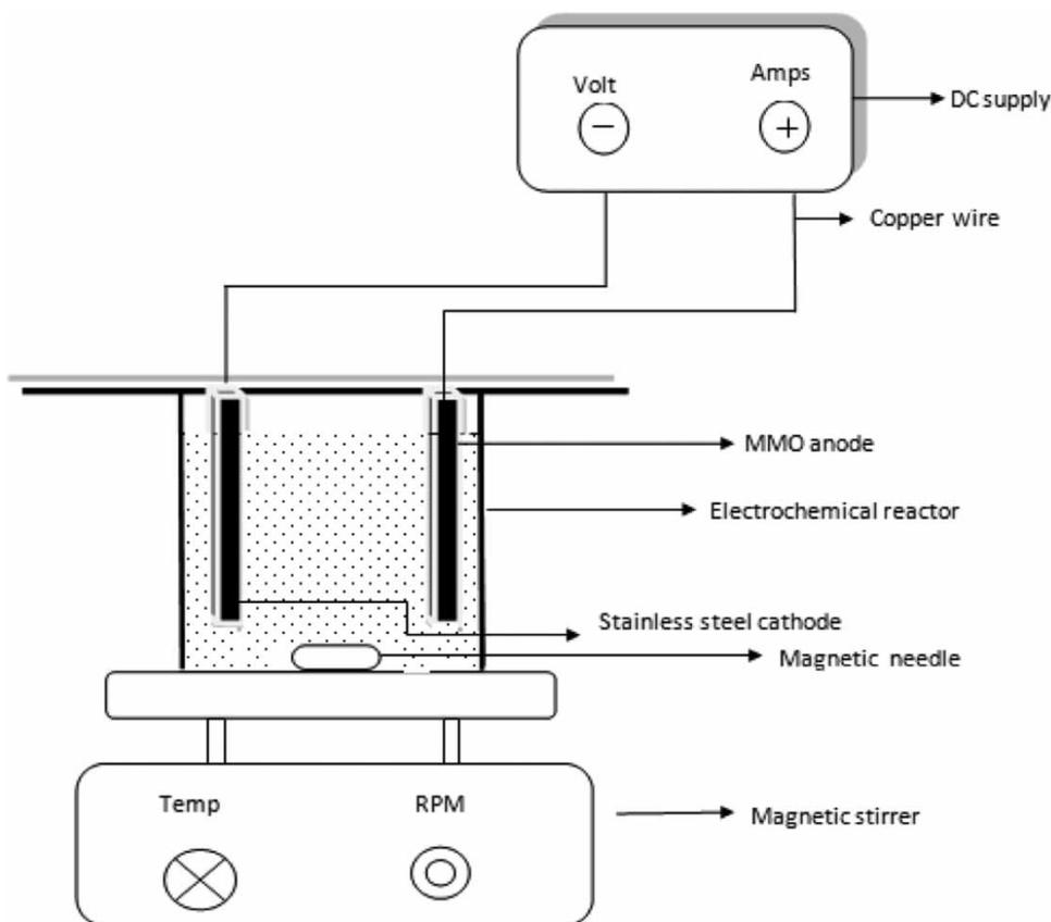
Figure 3 | Schematic diagram of the reactor set-up.
