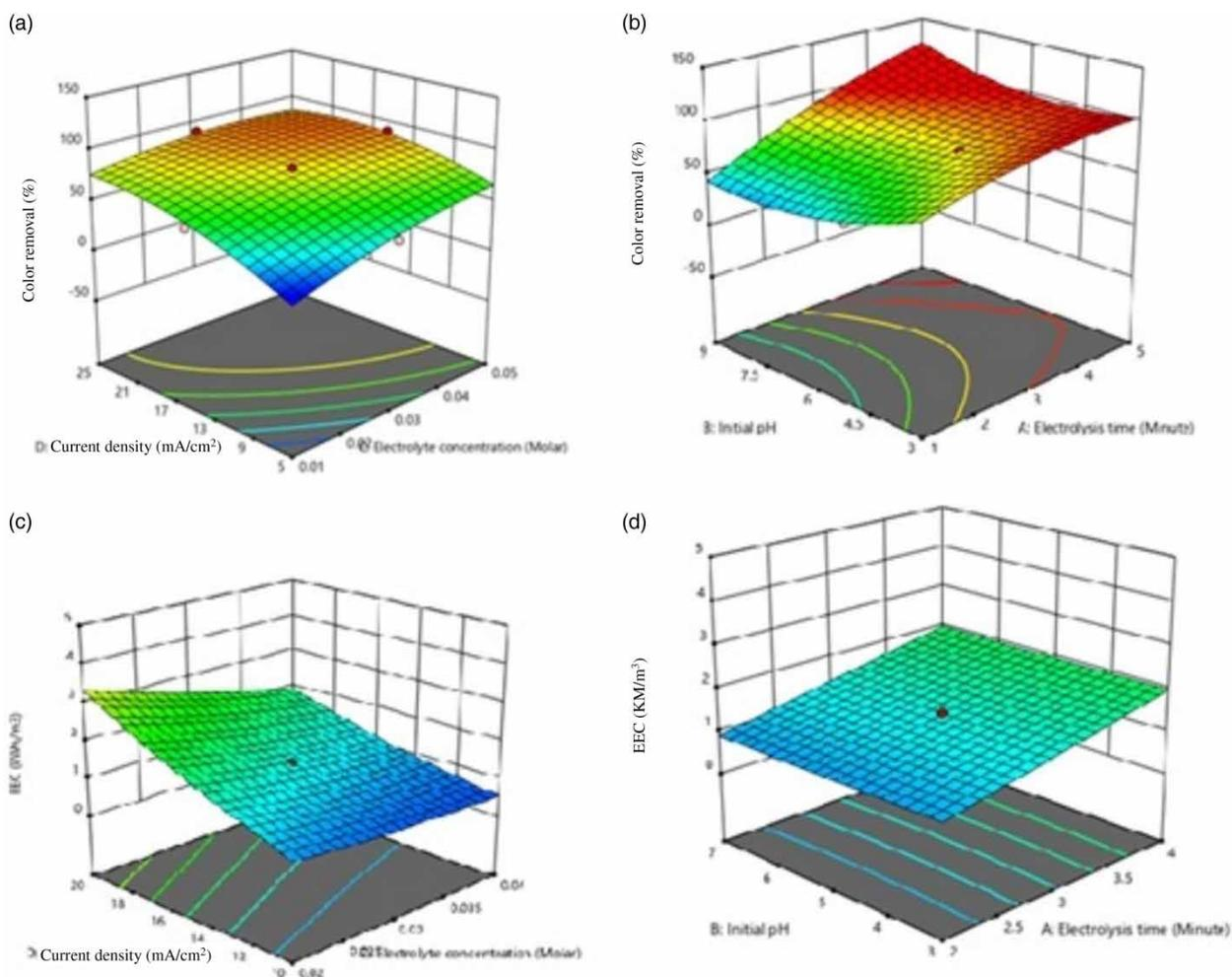
**Figure 8** | Response surface plot for effect of (a) current density with electrolyte concentration on color removal, (b) initial pH with electrolysis time on color removal, (c) current density with electrolyte concentration on energy consumption and (d) initial pH along with electrolysis time on energy consumption.
