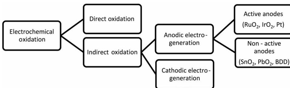
Figure 1 | Schematic electrochemical oxidation process.
