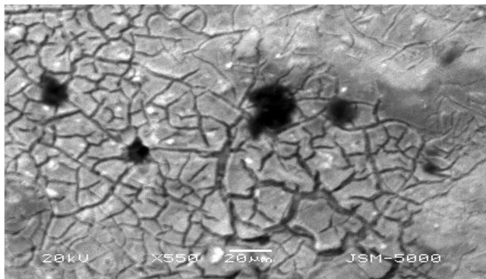
Figure 4 | SEM image of MMO electrode.
