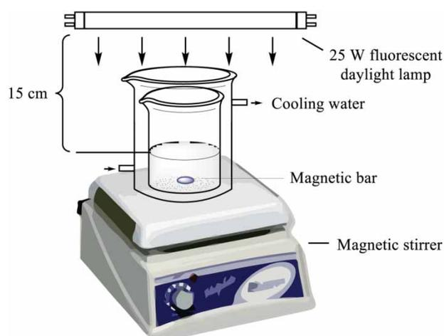
Figure 2 | Reactor of photocatalysis for DBP.
