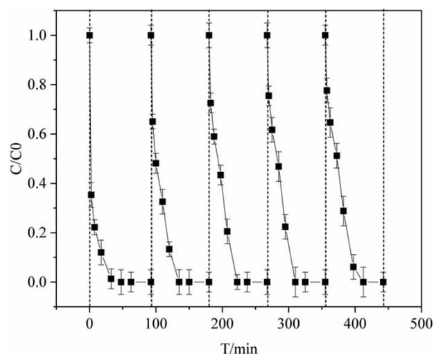
**Figure 9** | Repeated degradation and recovery of oxytetracycline by Vis/NGO-Fe<sub>3</sub>O<sub>4</sub>/PDS (initial OTC concentration = 50 mg L<sup>-1</sup>, PDS concentration = 1 mM, [NGO-Fe<sub>3</sub>O<sub>4</sub>]:[PDS] = 4:1, pH = 3.0, temperature = 20 ± 2 °C, xenon lamp (500 W/50 Hz)).
