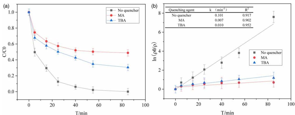
**Figure 8** | (a) The degradation of oxytetracycline under different quencher conditions, and (b) degradation kinetics of oxytetracycline under different quencher (initial OTC concentration = 50 mg L<sup>-1</sup>, PDS concentration = 1 mM, [NGO-Fe<sub>3</sub>O<sub>4</sub>]:[PDS] = 4:1, pH = 3.0, temperature = 20 ± 2 °C, xenon lamp (500 W/50 Hz)).
