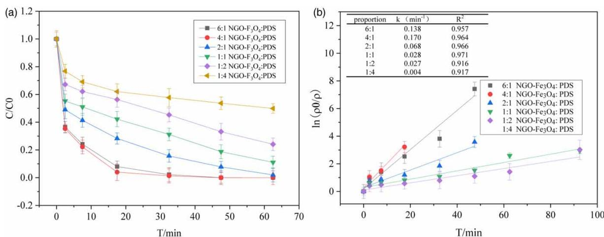
**Figure 5** | (a) The degradation of oxytetracycline under different ratio conditions, and (b) degradation kinetics of oxytetracycline under different ratio conditions (initial OTC concentration = 50 mg L<sup>-1</sup>, PDS concentration = 1 mM, [NGO-Fe<sub>3</sub>O<sub>4</sub>]: [PDS] = 6:1, 4:1, 2:1, 1:1, 1:2, 1:4, temperature = 20 ± 2 °C, xenon lamp (500 W/50 Hz)).
