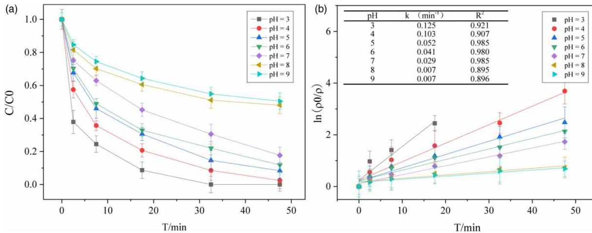
**Figure 6** | (a) The degradation of oxytetracycline under different pH conditions, and (b) degradation kinetics of oxytetracycline under different pH conditions (initial OTC concentration = 50 mg L<sup>-1</sup>, PDS concentration = 1 mM, [NGO-Fe<sub>3</sub>O<sub>4</sub>]:[PDS] = 4:1, pH = 3, 4, 5, 6, 7, 8, 9, temperature = 20 ± 2 °C, xenon lamp (500 W/50 Hz)).
