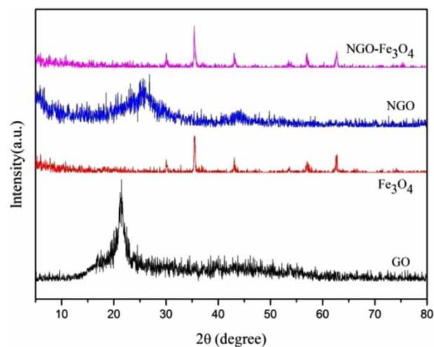
Figure 3 | XRD spectra of GO, NGO, Fe<sub>3</sub>O<sub>4</sub> and NGO-Fe<sub>3</sub>O<sub>4</sub>.
