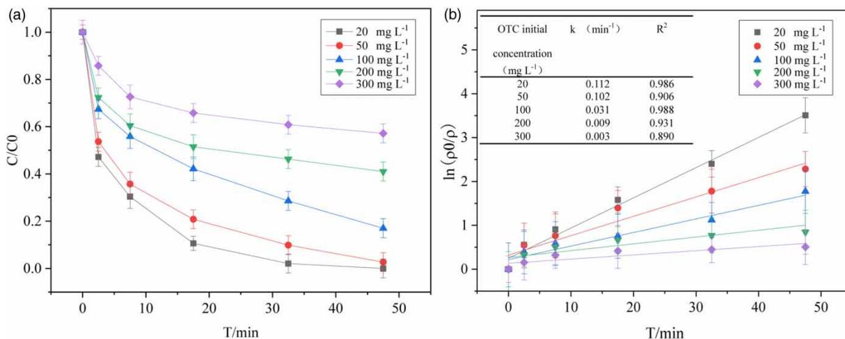
**Figure 7** | (a) The degradation of oxytetracycline under different initial concentration, and (b) degradation kinetics of oxytetracycline under different initial concentration (initial concentration = 20, 50, 100, 200, 300 mg L<sup>-1</sup>, PDS concentration = 1 mM, [NGO-Fe<sub>3</sub>O<sub>4</sub>]:[PDS] = 4:1, pH = 3.0, temperature = 20 ± 2 °C, xenon lamp (500 W/50 Hz)).
