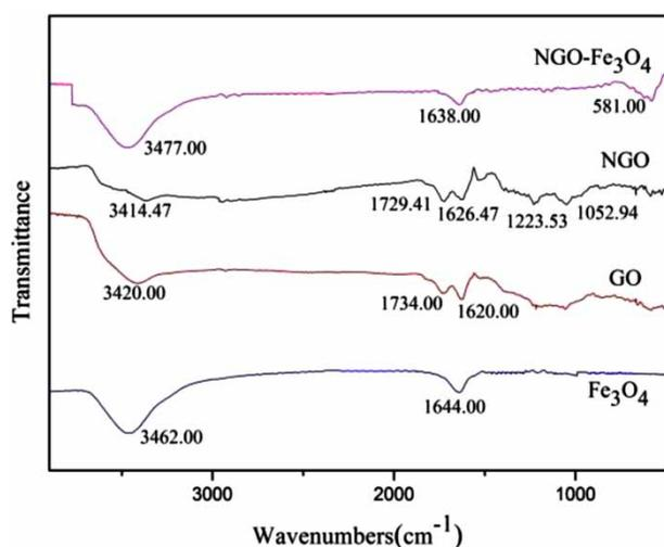
Figure 2 | FTIR spectra of GO, NGO, Fe<sub>3</sub>O<sub>4</sub> and NGO-Fe<sub>3</sub>O<sub>4</sub>.
