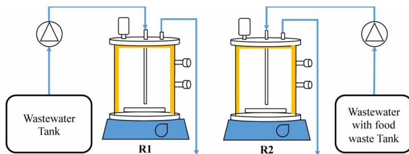
Figure 1 | Schematic of the laboratory-scale sewer reactor system. R1 without FW addition, R2 with FW addition.
