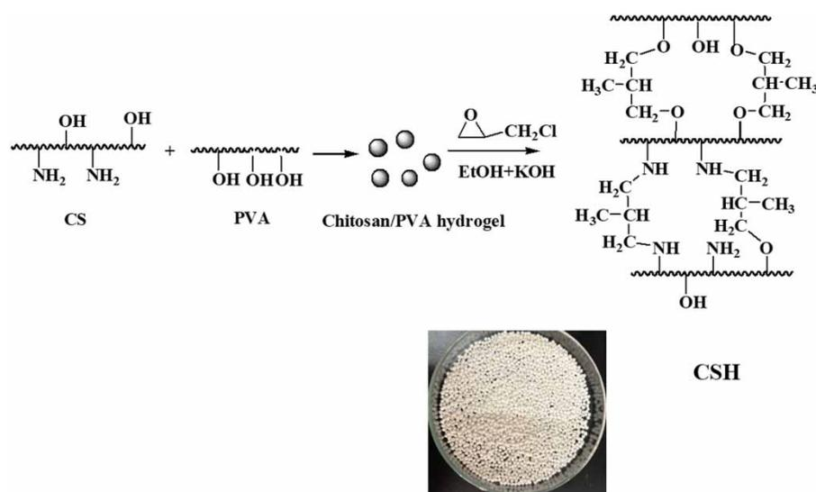
Figure 1 | Preparation scheme of CSH adsorbent.
