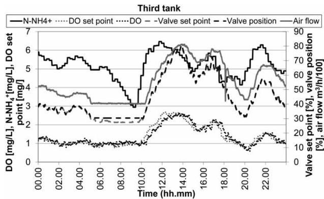
**Figure 1** | Typical behaviour of the fuzzy controller installed on the full-scale plant. Trends, over one day, of dissolved oxygen (DO) concentration and set point, N-NH<sub>4</sub><sup>+</sup> concentration, valve position (actual and set point), and air flow.
