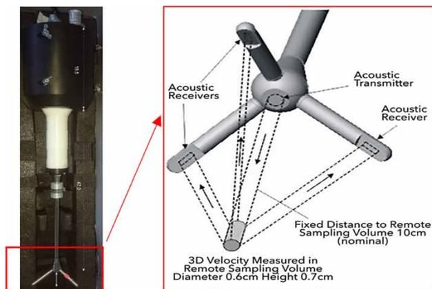
**Figure 3** | ADV device with the probes.
