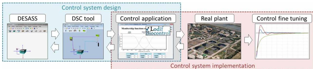
Figure 5 | Schematic representation of the development procedure for the controllers to be implemented in WWTPs.
