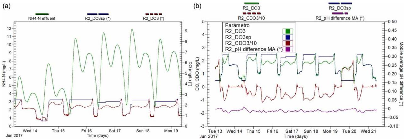
**Figure 6** | Evolution of: (a) DO set point (R2\_DO3sp) and ammonium concentration in the outlet of the aerobic reactor (NH4-N effluent). R2\_DO3 is the measured DO concentration in the reactor lane 2; and (b) inputs to the controller (Moving Average of pH difference (R2\_pH difference MA), cumulative DO error in the third aerated chamber over ten (R2\_CDO3/10), DO (R2\_DO3) and DO set point (R2\_DO3sp) in last aerated chamber).
