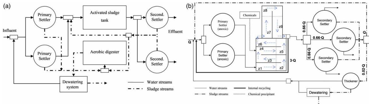
Figure 2 | Treatment scheme of Denia WWTP: (a) original, (b) upgraded.
