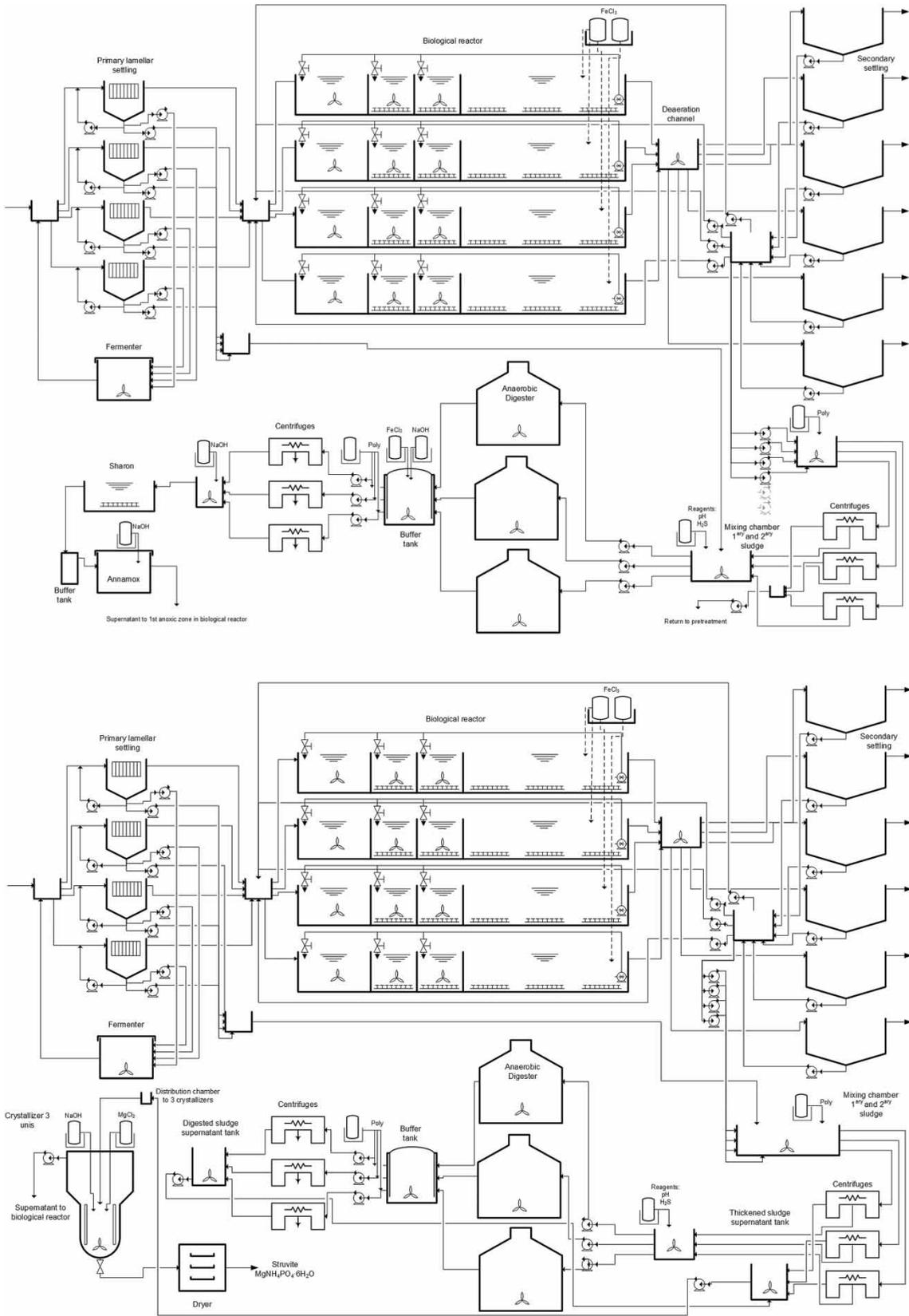
Figure 1 | Flow diagram of the base solution (above) and alternative solution (below).
