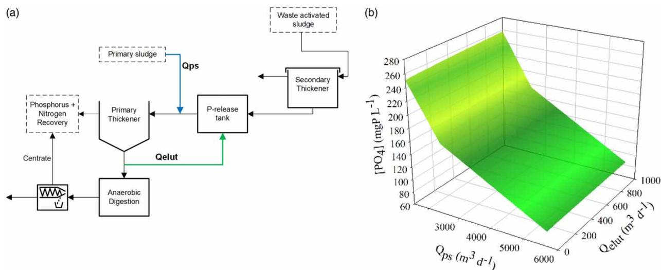
**Figure 3** | (a) Schematic representation of the sludge line configuration simulated (b) concentration of phosphorus in the primary thickener overflow at different operational conditions: primary sludge flow ( $Q_{ps}$ ) (blue line into the primary thickener) and elutriation flow ( $Q_{elut}$ ) (green line from the primary thickener to the P-release tank). The full colour version of this figure is available in the online version of this paper, at <http://dx.doi.org/10.2166/wst.2020.056>.
