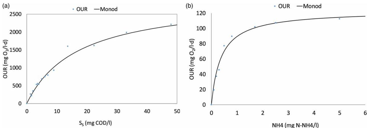
Figure 4 | OUR values obtained at different substrate concentrations for (a) heterotrophic bacteria, (b) autotrophic bacteria.
