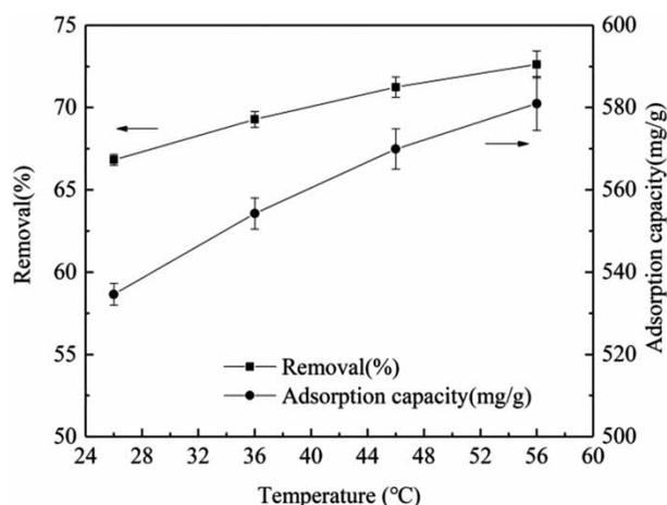
**Figure 10** | Effect of different temperatures on the adsorption of microplastics on 3D RGO.
