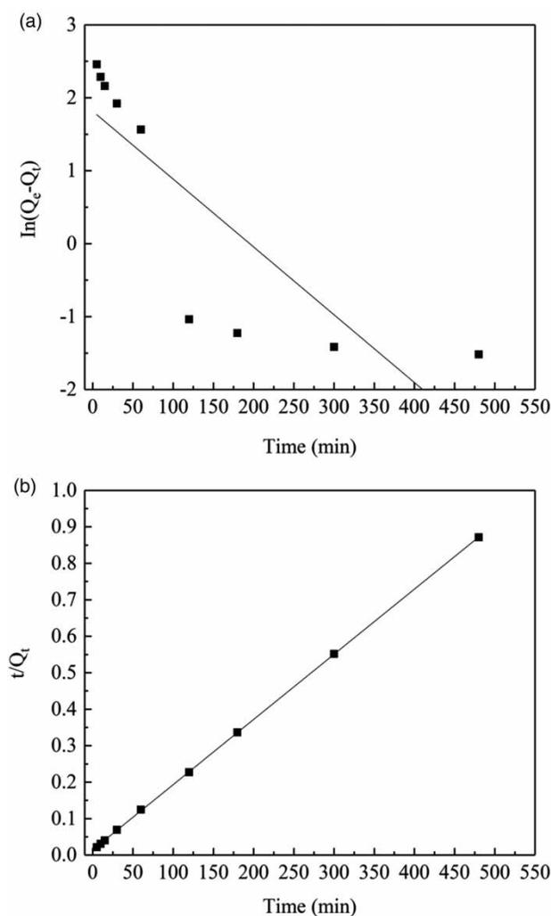
**Figure 9** | Adsorption kinetics of 3D RGO. (a) Pseudo-first-order kinetic model, (b) pseudo-second-order kinetic model.
