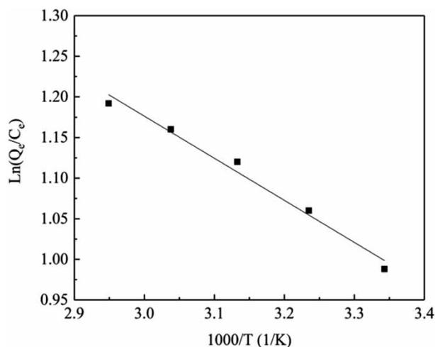
**Figure 11** | Plot of  $\ln(Q_e/C_e)$  versus  $1/T$ .
