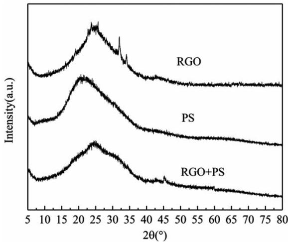
**Figure 7** | XRD patterns of 3D RGO, PS microplastics, and 3D RGO after adsorption.
