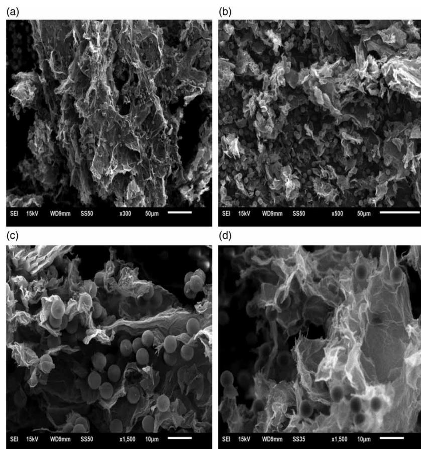
**Figure 6** | SEM images of 3D RGO after adsorption, magnified (a) 300 times, (b) 500 times, (c) 1,500 times, and (d) 1,500 times.
