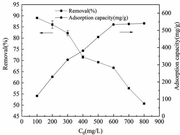
**Figure 4** | Effect of different initial concentrations on the adsorption of PS microplastics on 3D RGO.
