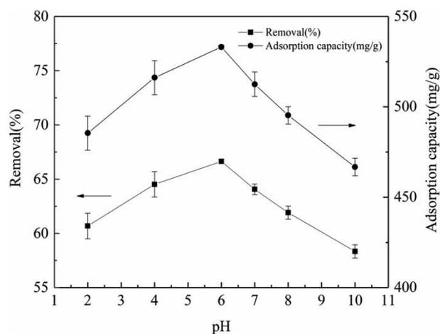
Figure 1 | Effect of different initial pH values on the adsorption of microplastics on 3D RGO.
