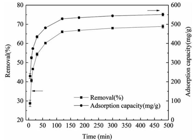
**Figure 8** | Effect of different adsorption time on the adsorption of PS microplastics on 3D RGO.
