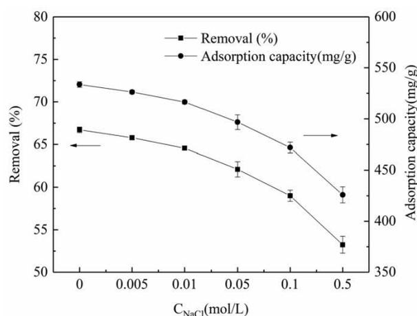
Figure 3 | Effect of different ion concentrations on the adsorption of PS microplastics on 3D RGO.
