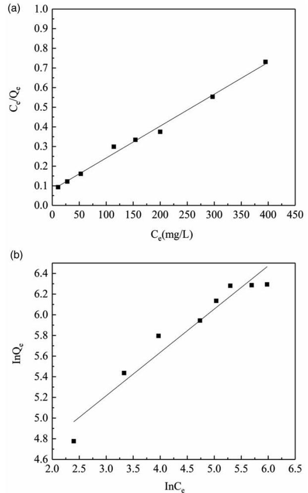
**Figure 5** | Adsorption isotherms of 3D RGO. (a) Langmuir adsorption isotherm, (b) Freundlich adsorption isotherm.
