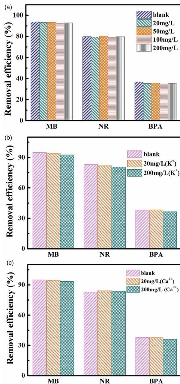
**Figure 7** | Effect of concentrations of coexisting FA (a),  $Ca^{2+}$  (b) and  $K^+$  (c) on the removal efficiencies of MB, NR and BPA. Solution volume: 50 mL, adsorbent dosage: 1 g/L, contaminant concentration: 50 mg/L, temperature: 25 °C, initial pH: 6.0.
