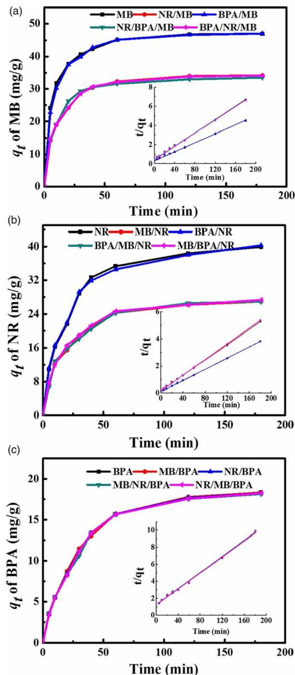
**Figure 6** | Adsorption kinetics of MB (a), NR (b) and BPA (c) by PDA-CD polymers in the single and tandem system. Insets: adsorption kinetics fitted by pseudo-second order kinetic model. Contaminant concentration: 50 mg/L, solution volume: 100 mL, adsorbent dosage: 1 g/L, initial pH: 6, temperature: 25°C.
