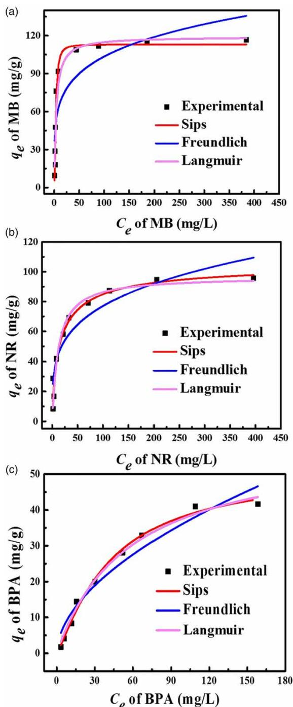
**Figure 4** | Adsorption isotherms of pollutants by PDA-CD polymers (a: MB, b: NR, c: BPA) and model fitting.
