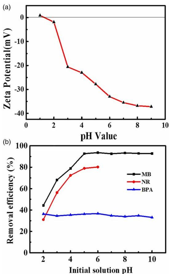
**Figure 3** | (a) Effect of initial solution pH on the Zeta potentials of PDA-CD. Volume of deionized water: 10 mL, amount of polymers: 50 mg, temperature: 25 °C. (b) Effect of initial solution pH on the adsorption. Contaminant concentration: 50 mg/L, solution volume: 50 mL, adsorbent dosage: 1 g/L, temperature: 25 °C.
