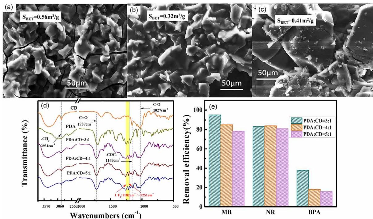
**Figure 2** | The SEM image and BET data of PDA-CD polymers: (a) PDA:CD = 3:1; (b) PDA:CD = 4:1; (c) PDA:CD = 5:1. (d) The FT-IR spectra of CD and PDA-CD polymers with different ratios. (e) Adsorption of MB, NR and BPA by PDA-CD polymers with different molar ratios.
