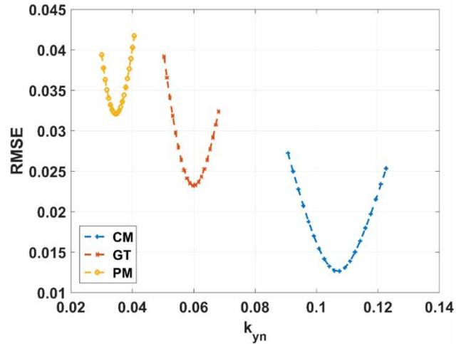
**Figure 7** | Parameter sensitivity analysis for Clark's model parameters ( $A$  and  $r$ ) for the adsorption of Co (II) ions on chamomile (CM), green (GT) and peppermint (PM) tealeaves.
