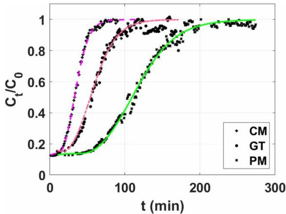
**Figure 6** | Breakthrough curve for Co (II) ion adsorption on a fixed-bed column experiment using spent tealeaves. The symbols represent data points, the lines represent model simulations using the Thomas model.
