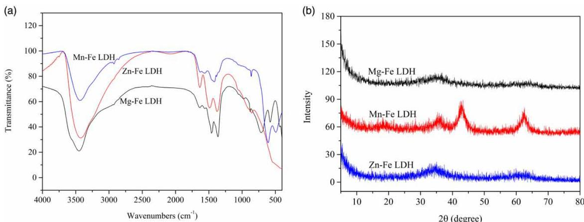
**Figure 3** | The FT-IR spectrum (a) and XRD (b) of Mg-Fe LDH, Zn-Fe LDH, and Mn-Fe LDH (the molar ratio of M/Fe = 3:1).
