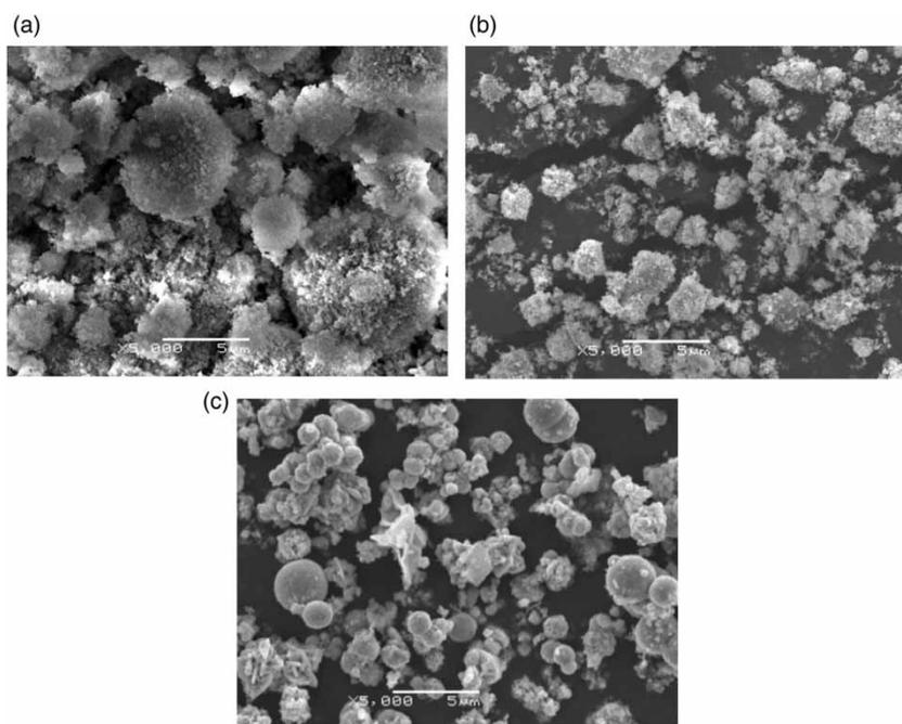
**Figure 2** | SEM image of M-Fe LDH adsorbent: (a) Mg-Fe LDH; (b) Zn-Fe LDH; (c) Mn-Fe LDH.
