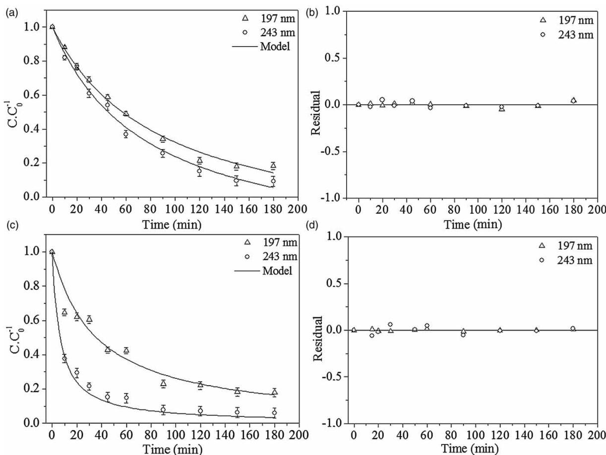
**Figure 3** | Kinetic evaluation of paracetamol degradation by photo-Fenton/LED and photo-Fenton/UV-C systems: (a) and (c) adjusting the kinetic model; (b) and (d) residual graphs, respectively.
