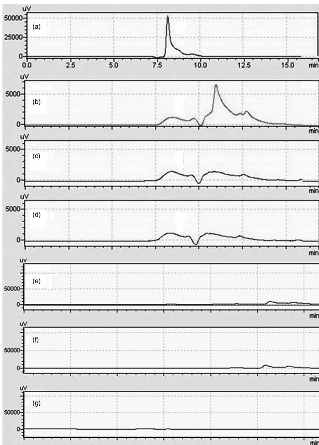
**Figure 5** | Chromatograms of the paracetamol solution: (a) before treatment; after photo-Fenton/LED: (b) 60 min, (c) 120 min and (d) after 180 min; after photo-Fenton/UV-C: (e) 60 min, (f) 120 min and (g) 180 min.
