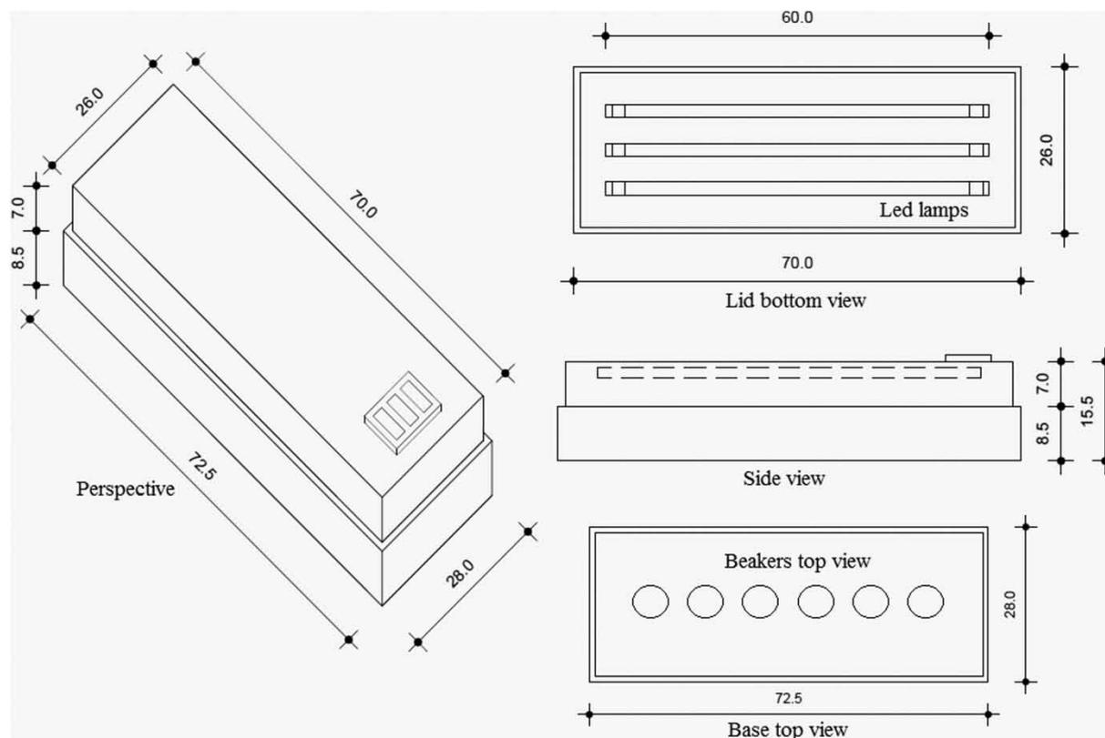
Figure 2 | Schematic drawing of the LED photo-reactor (measurements in cm).
