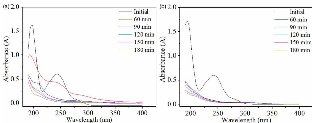
**Figure 4** | Spectral monitoring of kinetics degradation by systems: (a) photo-Fenton/LED and (b) photo-Fenton/UV-C.
