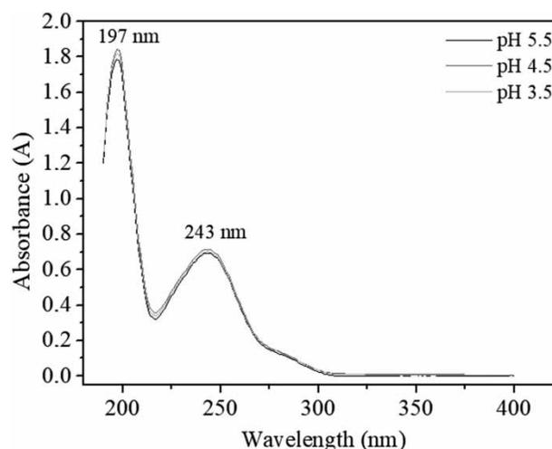
Figure 1 | Spectral scanning of paracetamol solution at different pH.
