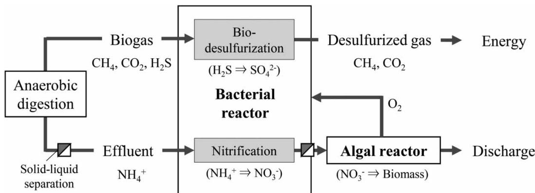
**Figure 1** | A proposed coupling process of biogas desulfurization and effluent nutrients removal after anaerobic digestion using aerobic bacterial reactor and microalgal reactor.
