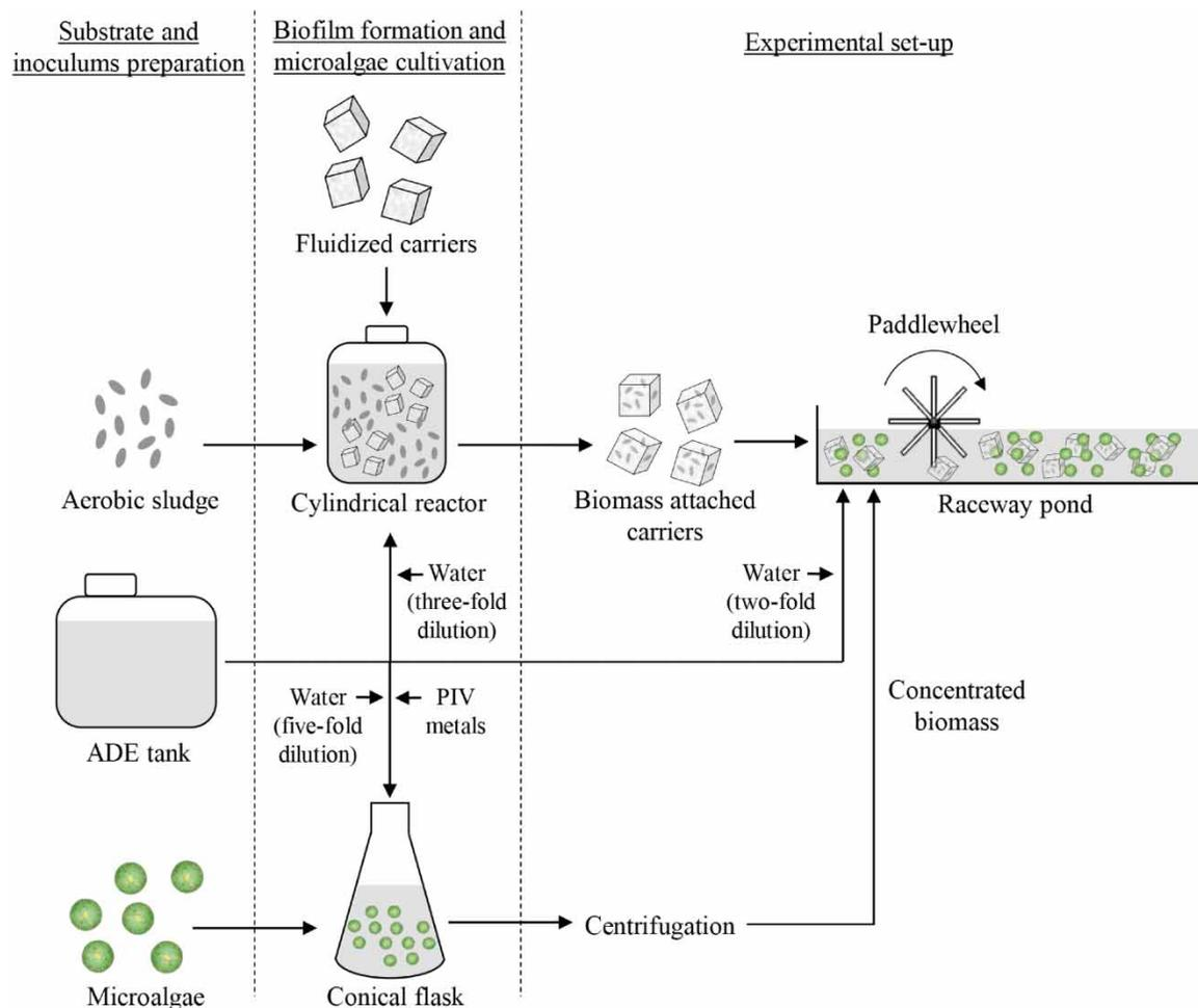
**Figure 1** | A schematic diagram of a series of experimental procedures. Bacterial inoculum for the raceway pond also includes suspended form.
