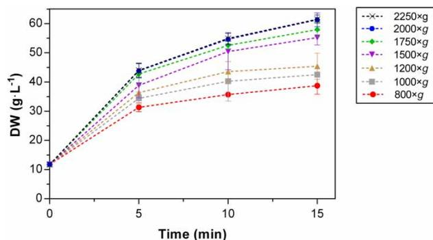
**Figure 3** | Microalgae concentration evaluation, expressed as dry weight (DW), using different centrifugal forces and centrifugation times. The initial DW of  $11.8 \pm 0.2 \text{ g}\cdot\text{L}^{-1}$  was obtained in the sedimentation tests at the optimal conditions (pH 12,  $G_V = 250 \text{ s}^{-1}$ , and  $T_M = 10$  seconds).
