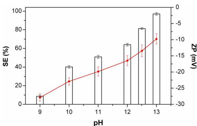
**Figure 1** | Effect of pH value on sedimentation efficiency (SE) of *Chlorella sorokiniana* (bars) and on zeta potential measurements (ZP, red line). Tests were carried out using  $G_V = 500 \text{ s}^{-1}$  and  $T_M = 10$  seconds. ZP measurements were taken immediately after the coagulation process for each condition. Please refer to the online version to see this figure in color: <http://dx.doi.org/10.2166/wst.2020.106>.
