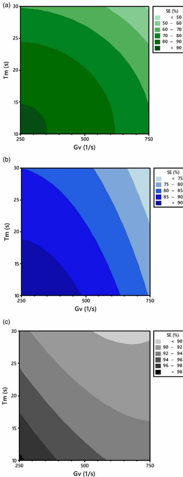
**Figure 2** | Variation of sedimentation efficiency (SE) of *Chlorella sorokiniana* using different values of mixing times ( $T_M$ ) and velocity gradient ( $G_V$ ) at pH (a) 12, (b) 12.5, and (c) 13. Please refer to the online version to see this figure in color. <http://dx.doi.org/10.2166/wst.2020.106>.
