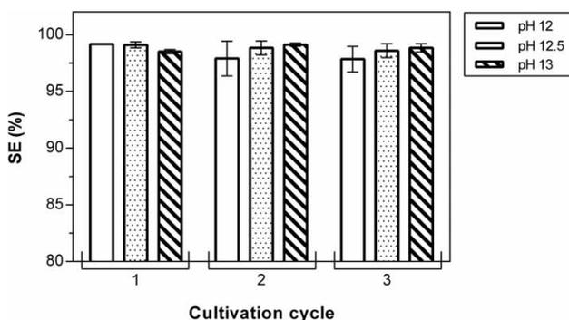
**Figure 5** | Sedimentation efficiencies (SEs) of *Chlorella sorokiniana* using three different photobioreactor effluents (PBREs). The tests were carried out using the optimized parameters ( $G_V = 250 \text{ s}^{-1}$  and  $T_M = 10$  seconds).
