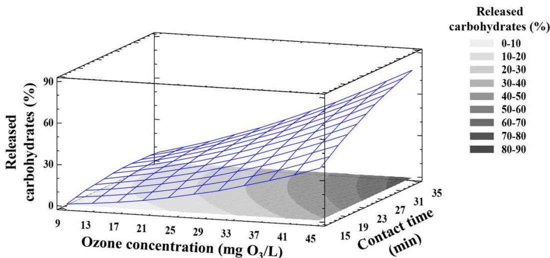
**Figure 1** | Response surface of released carbohydrates as a function of contact time and ozone concentration (pH 11). Triplicate measurements ( $n = 3$ ) are shown for each data set.
