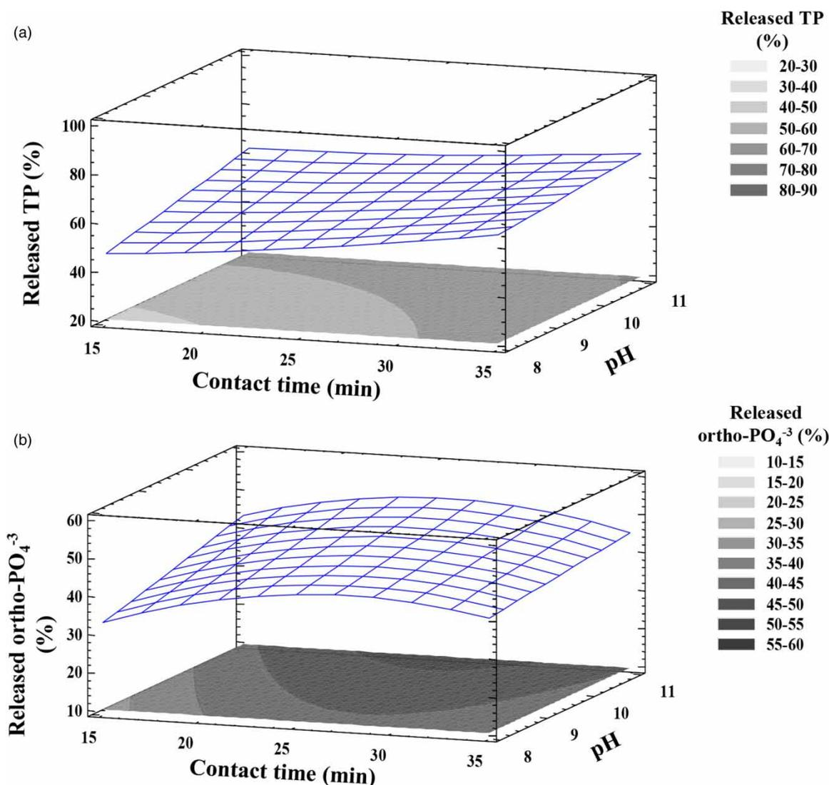
**Figure 3** | Response surface of released TP and ortho- $\text{PO}_4^{3-}$  as a function of pH and contact time (27 mg  $\text{O}_3/\text{L}$  ozone concentration). Triplicate measurements ( $n = 3$ ) are shown for each data set.
