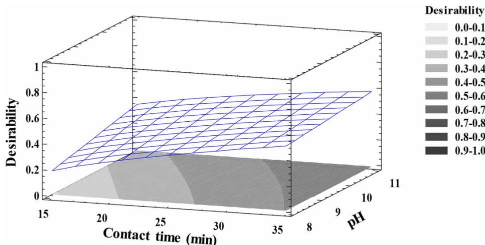
Figure 5 | Response surface for desirability function of ozone pretreatment as a function of pH and contact time. Triplicate measurements ( $n = 3$ ) are shown for each data set.
