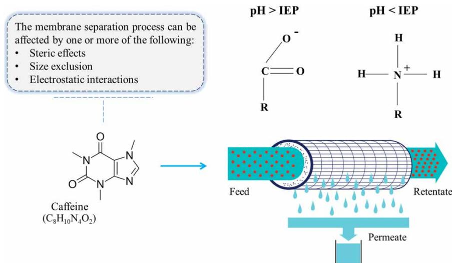
Figure 2 | Effect of feed solution pH on the functional groups on the surface of the membrane. Source: Rigueto *et al.* (2020).
