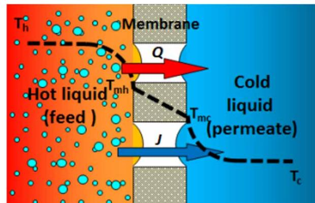
Figure 11 | Basic principles of MD process. Source: Ghaffour *et al.* (2013).
