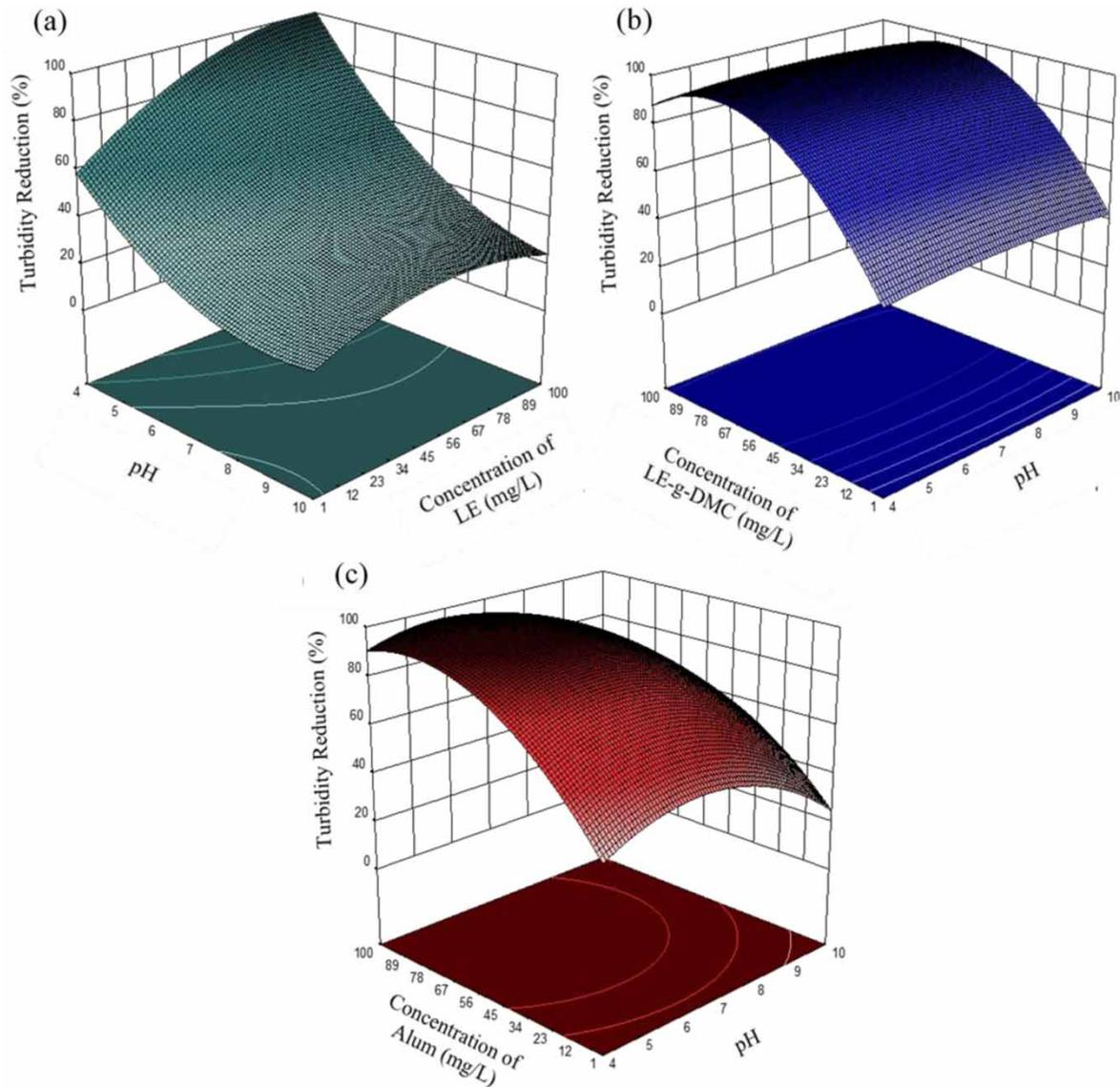
**Figure 1** | Three-dimensional response surface plots of the effect of pH and concentration of coagulants for turbidity removal (%) using (a) LE, (b) LE-g-DMC and (c) alum as coagulants in agriculture wastewater treatment.
