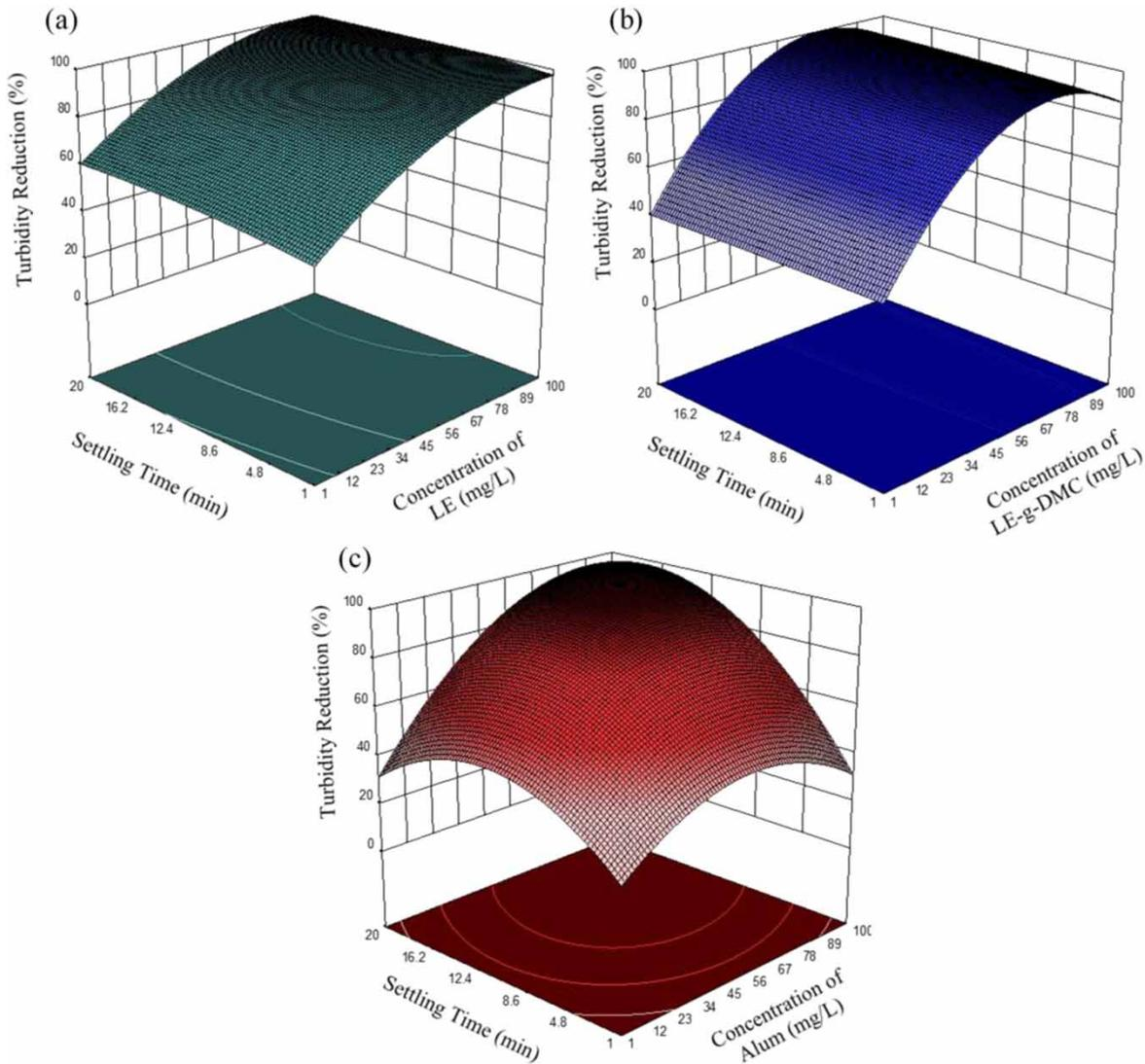
**Figure 5** | Three-dimensional response surface plots of the effect of concentration of coagulants and settling time for turbidity removal (%) by using (a) LE, (b) LE-g-DMC and (c) alum as coagulants in agriculture wastewater treatment.
