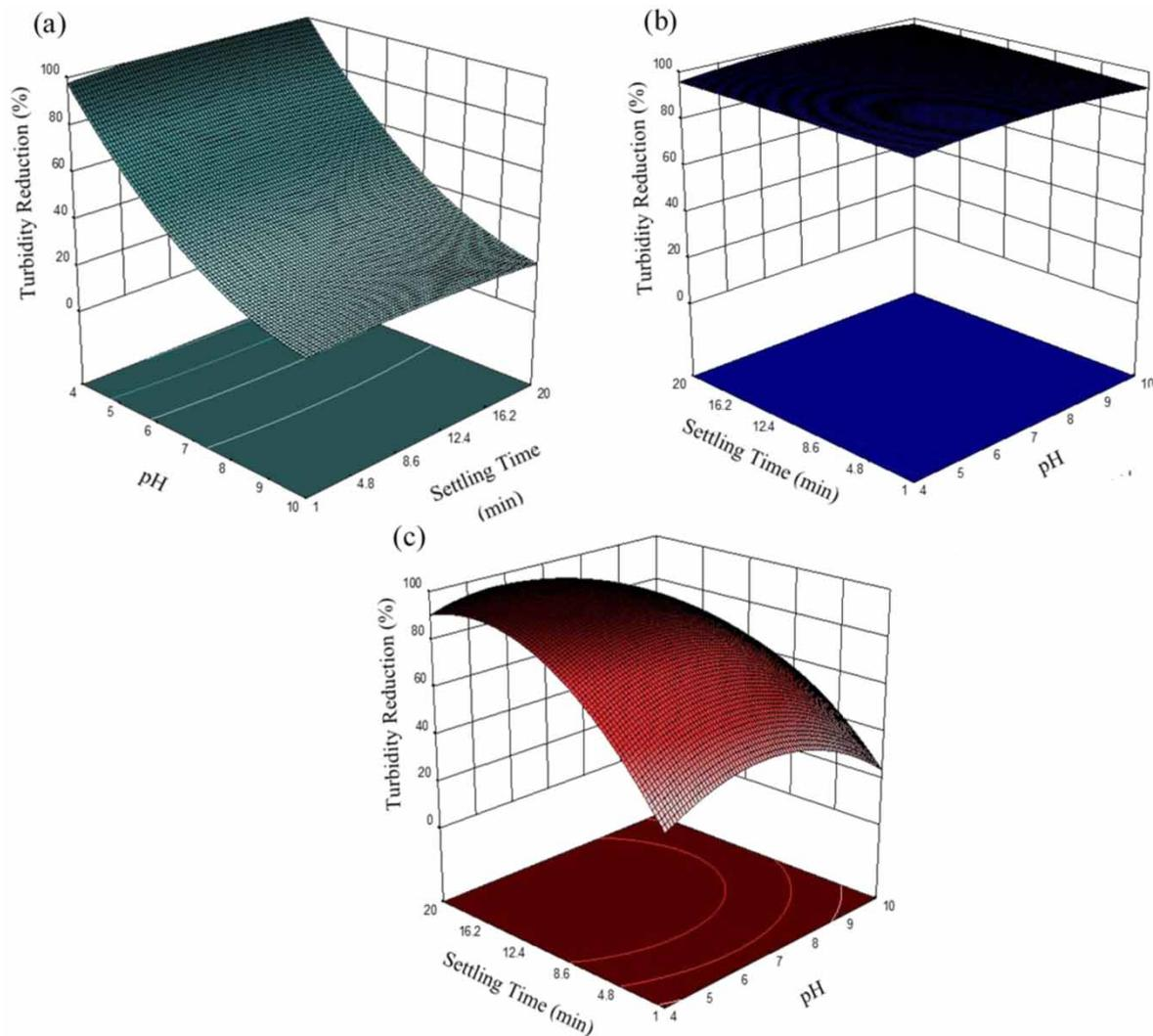
**Figure 3** | Three-dimensional response surface respond plots of the effect of pH and settling time for turbidity removal (%) using (a) LE, (b) LE-g-DMC and (c) alum as coagulants in agriculture wastewater treatment.
