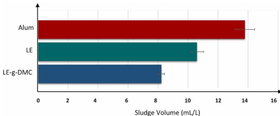
**Figure 7** | Sludge generated after the agriculture wastewater treatment.**Table 4** | Cost of LE, LE-g-DMC and alum in agricultural wastewater treatment
