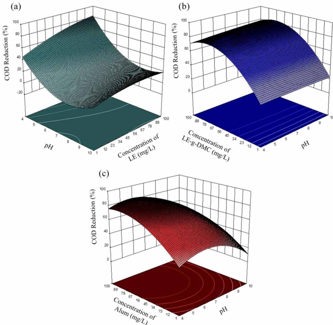
**Figure 2** | Three-dimensional response surface plots of the effect of pH and concentration of coagulants for COD removal (%) using (a) LE, (b) LE-g-DMC and (c) alum as coagulants in agriculture wastewater treatment.
