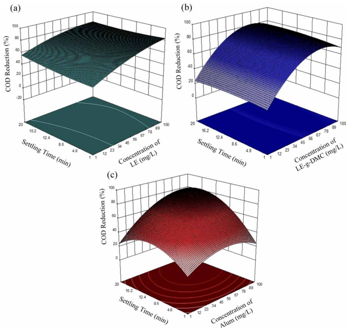
**Figure 6** | Three-dimensional response surface plots of the effect of concentration of coagulants and settling time for COD removal (%) by using (a) LE, (b) LE-g-DMC and (c) alum as coagulants in agriculture wastewater treatment.
