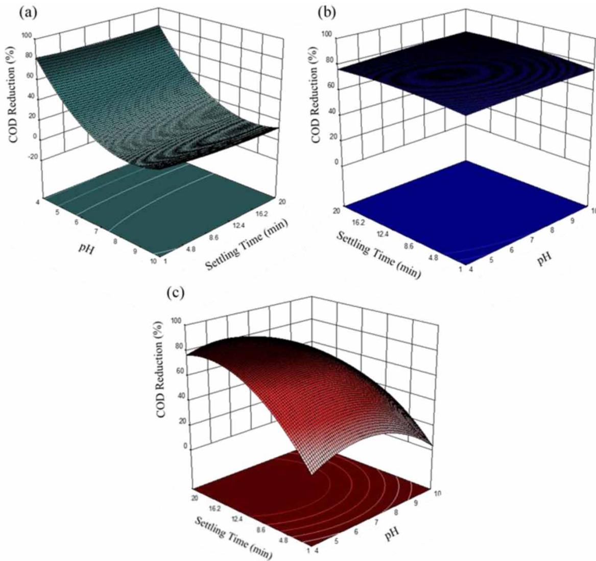
**Figure 4** | Three-dimensional response surface plots of the effect of pH and settling time for COD removal (%) using (a) LE, (b) LE-g-DMC and (c) alum as coagulants in agriculture wastewater treatment.
