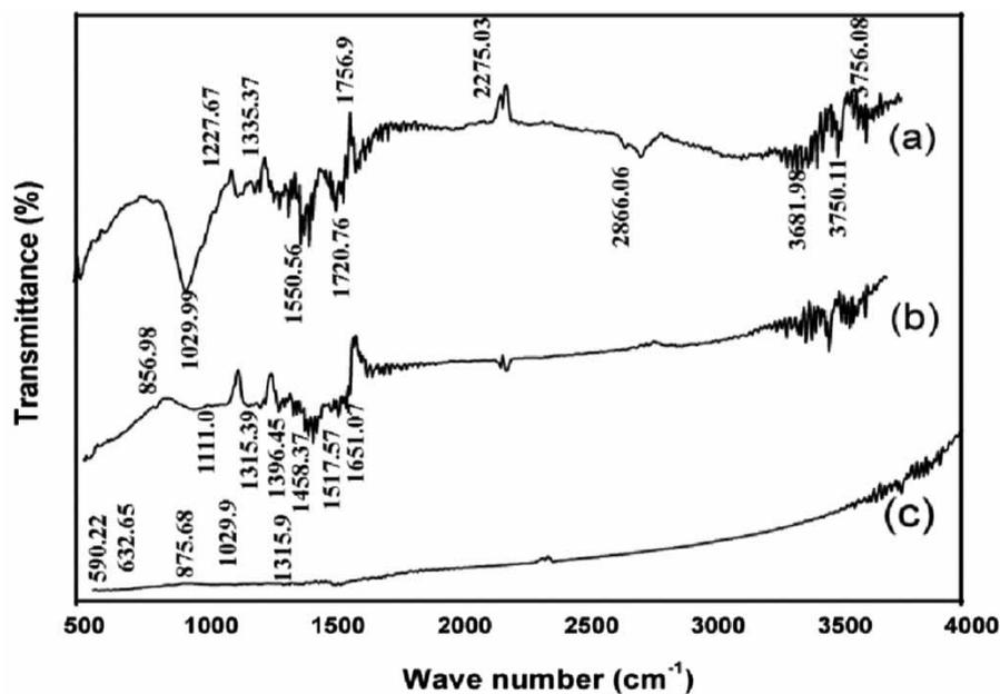
**Figure 3** | FTIR spectra of (a) BNH, (b) BNH-AC, and (c) BNH-AC after adsorption.
