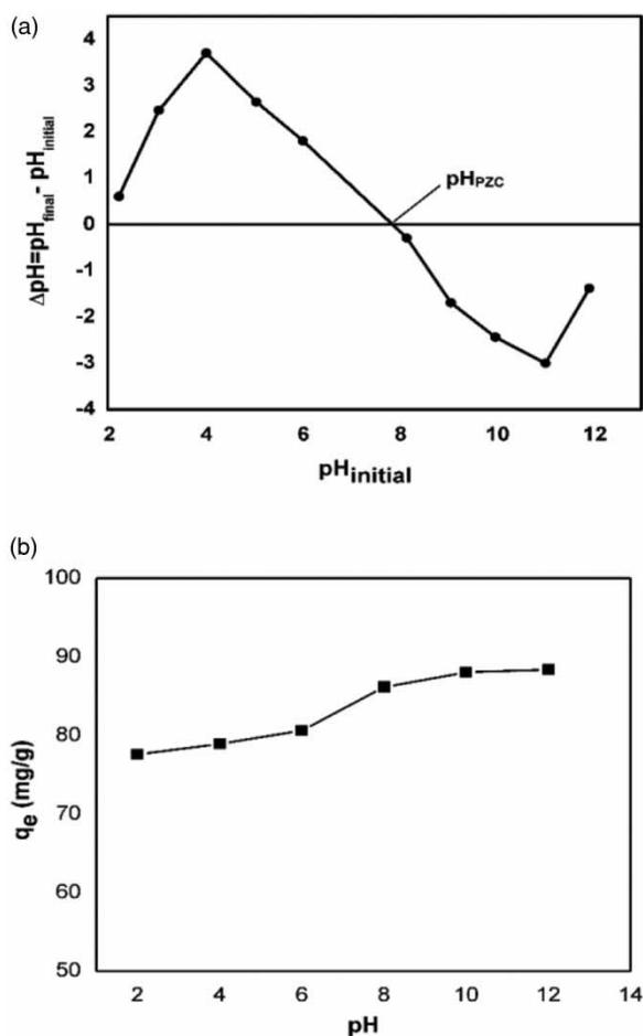
Figure 5 | (a)  $pH_{pzc}$  of BNH-AC, (b) effect of pH on MB removal by BNH-AC at 40 °C.
