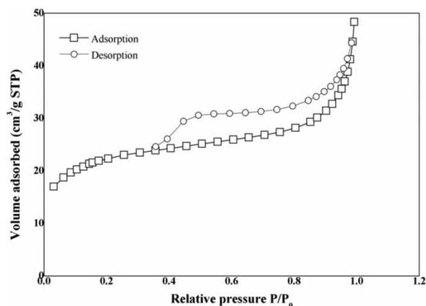
**Figure 1** | N<sub>2</sub> adsorption-desorption isotherms of BNH-AC.
