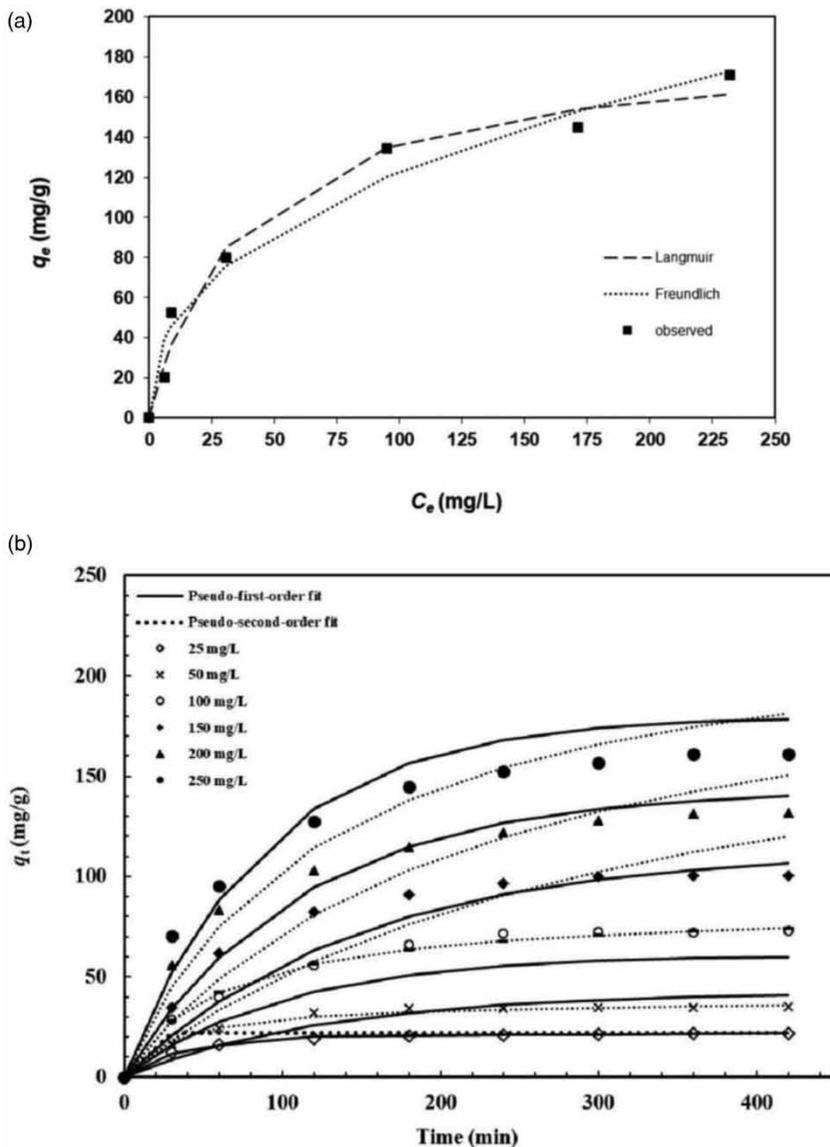
**Figure 6** | (a) Adsorption isotherm curve of the Langmuir and Freundlich models, (b) non-linear plots of the pseudo-first- and pseudo-second-order kinetic models for MB adsorption on BNH-AC at 40 °C.
