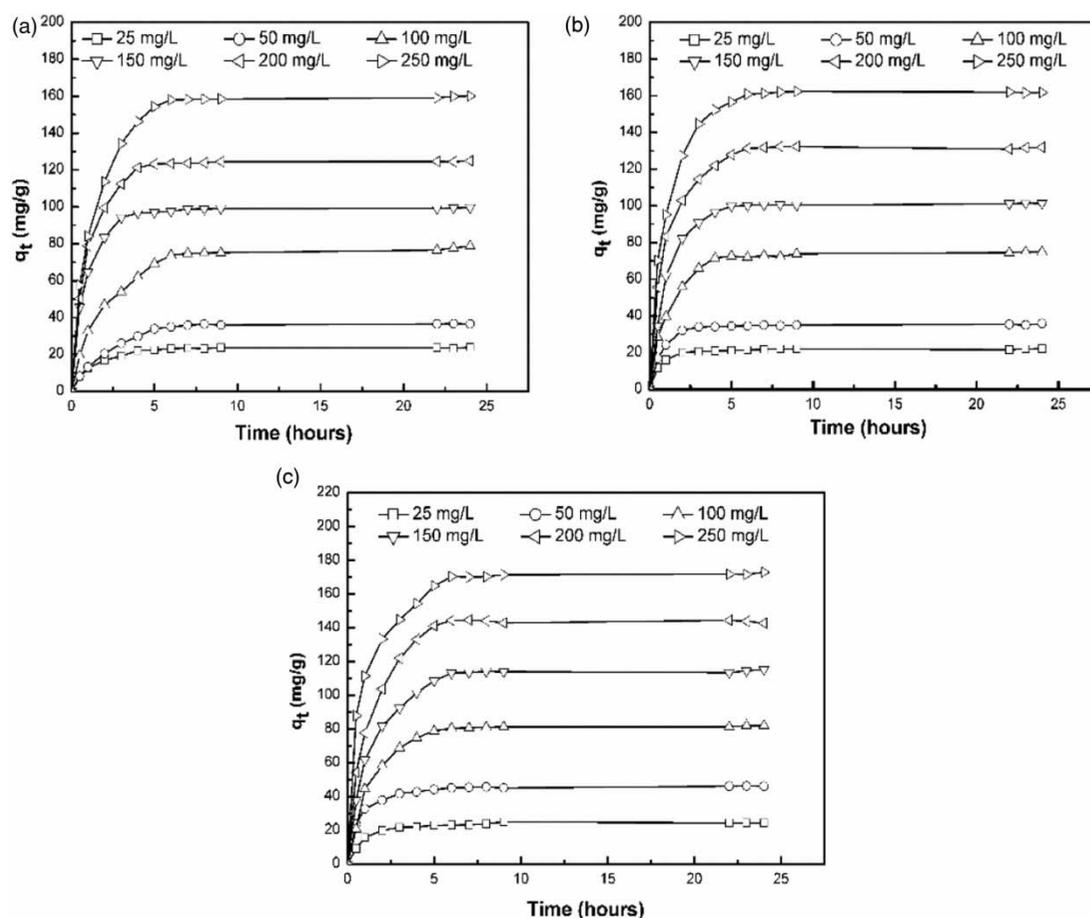
**Figure 4** | Effect of contact time on adsorption capacity ( $q_t$ ) of BNH-AC in different initial concentrations at (a)  $30\text{ }^\circ\text{C}$ , (b)  $40\text{ }^\circ\text{C}$  and (c)  $50\text{ }^\circ\text{C}$  (pH: 6.72, dose: 0.2 g).
